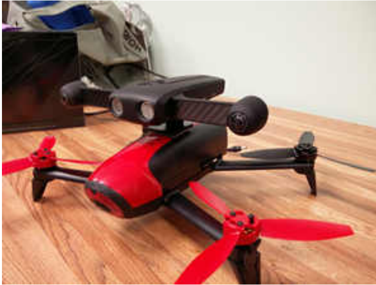
Figure 3.1. The system setup - A S.L.A.M.dunk mounted on a Parrot Bebop 2 drone
