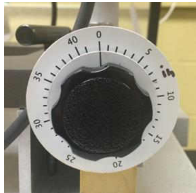
Figure 5.2: Dial used for introducing misalignment.
