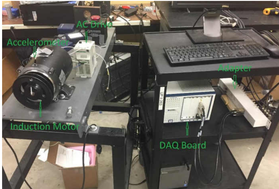
Figure 3.1: The experiment setup for obtaining vibration data.
