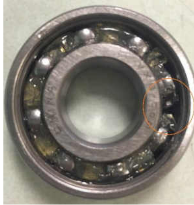
Figure 3.11: The damaged bearing
