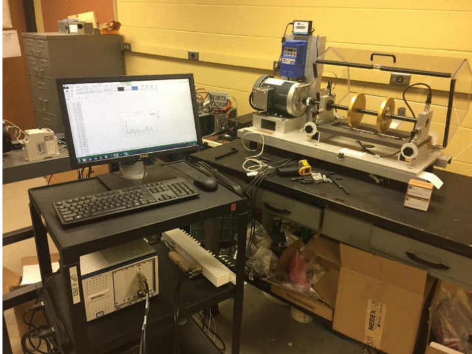
Figure 3.3: Machinery fault simulator used as third condition monitoring setup.
