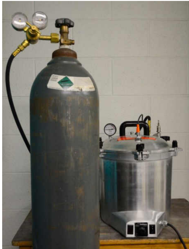
Figure 1: Carbonation Chamber Setup
