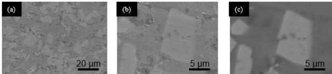
Figure 2.3. Secondary Electron images of Al(80)-Ti 3 SiC 2 (20) composites at, (a) low, and (b) higher magnification and (c) BSE image of the higher magnification region.
