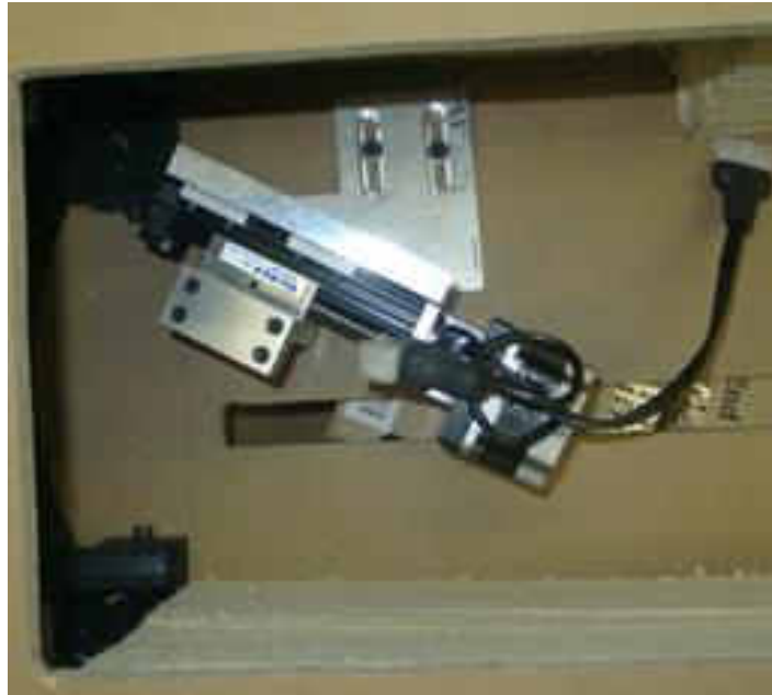
Figure 15. Traversing equipment mounted in test apparatus.
