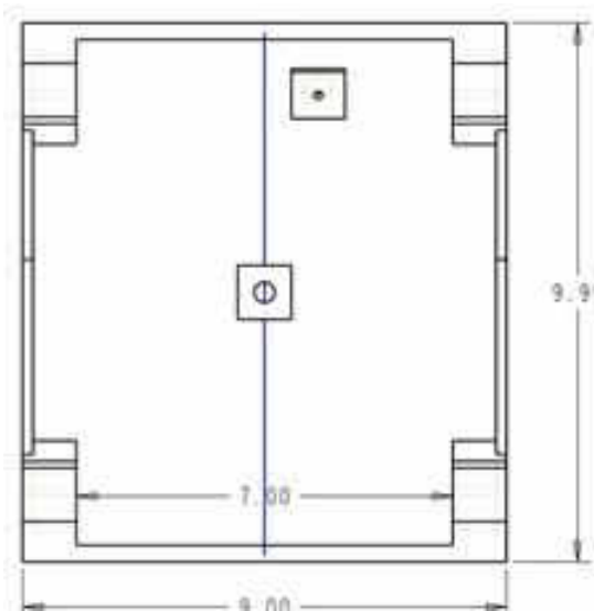
Figure 9. Back of cylinder tip (hole offsets).
