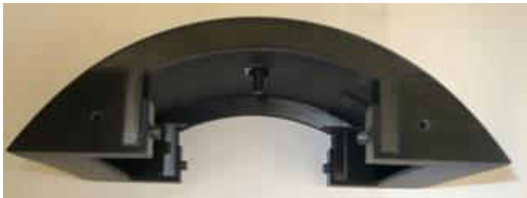
Figure 7. The assembled 0.4064 meter cylindrical leading edge tip.
