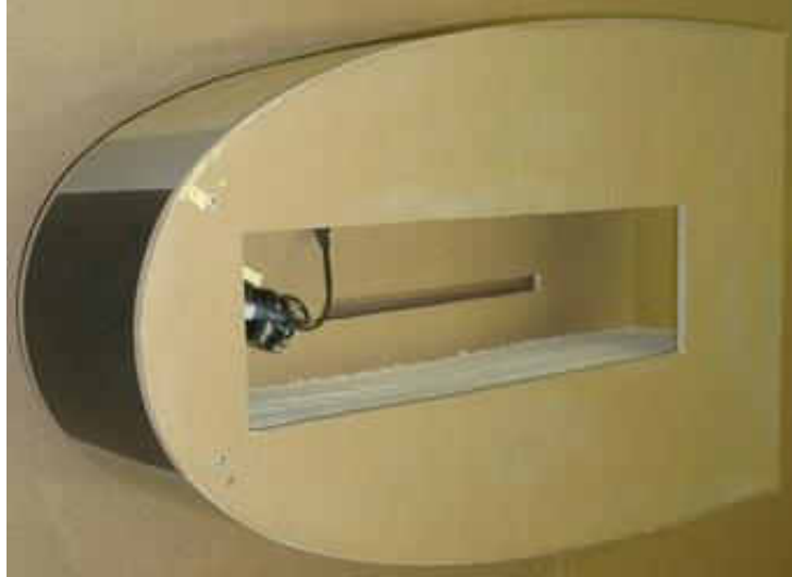
Figure 6. The 0.4064 meter cylindrical leading edge vane.
