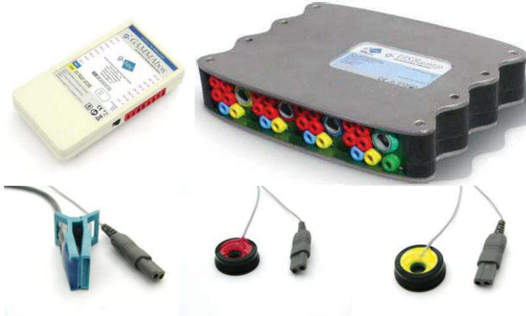
Figure 2.2 (top left) g.GAMMAbox, (top right) g.GAMMAusb, (bottom left) g.GAMMAearclip, (bottom middle) g.LADYbird, (bottom right) g.LADYbirdGND
