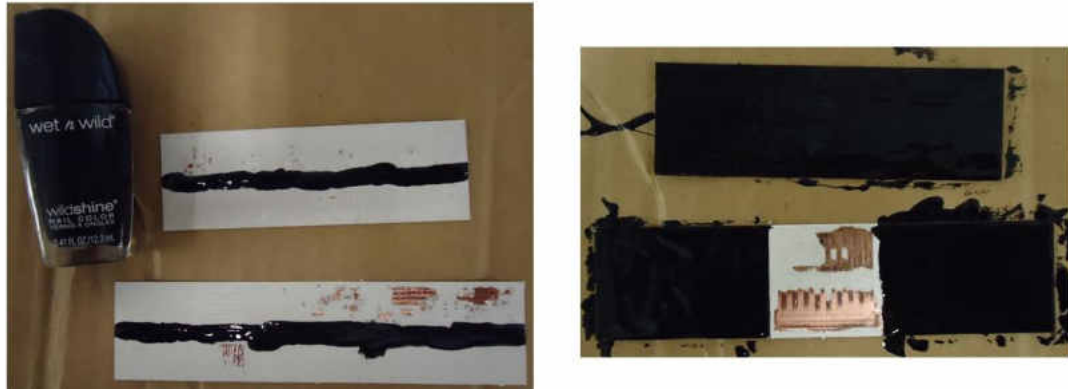
Figure 97. Finger nail polish applied to the PCB design.
