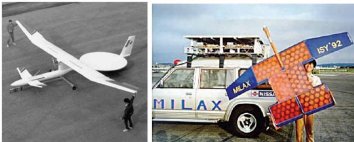
Figure 10. Model aircraft designed to utilize microwaves as their source of power. Figure on left is SHARP; and figure on right is MILAX.
