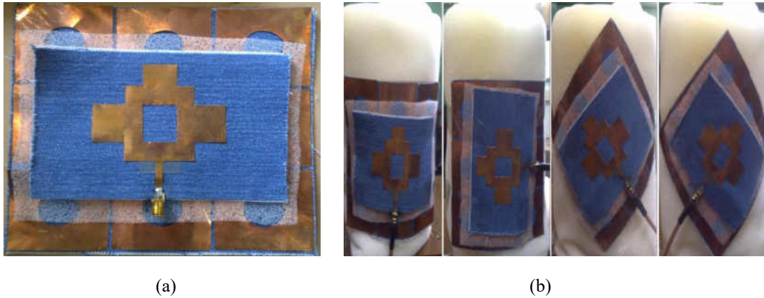
Fig. 2.4: (a) Fabricated prototype and (b) antenna under bending conditions [40].
