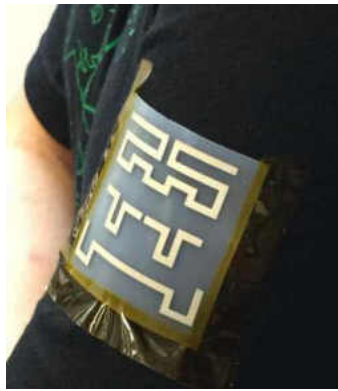
Fig. 2.5: Flexible antenna mounted on the human chest [43].
