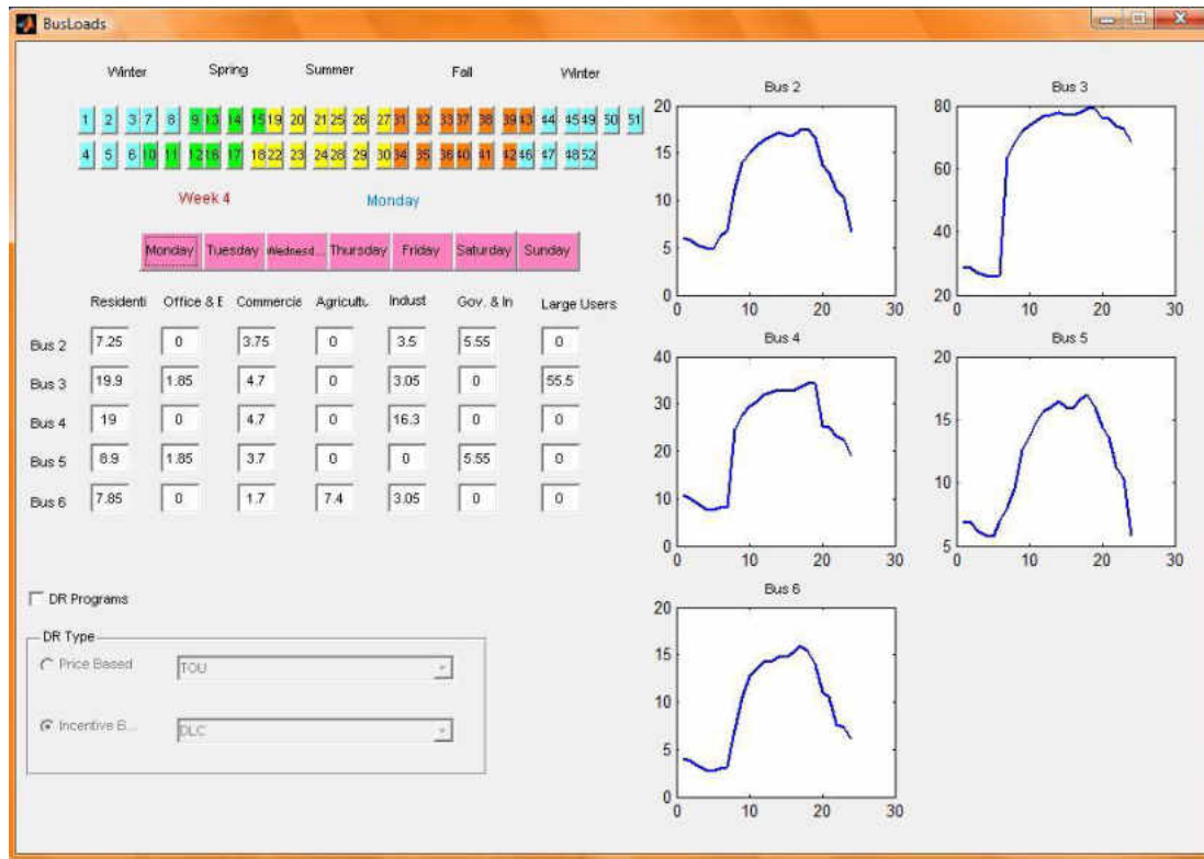
Figure 105. DR control panel showing loads on RBTS buses.
