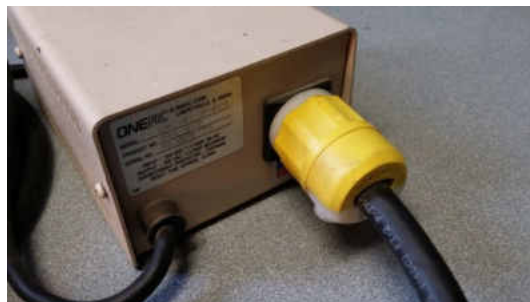
Figure 48. Isolation Transformer used for System Separation and Equipment Protection.
