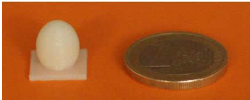
Figure 12. Fabricated lens antenna using AM [73].
