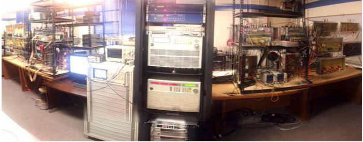
Figure 6.1: Hardware side of AC microgrid in the P-MG showing the inverters, filters, lines and power sources. The controller computers are located on the other side.
