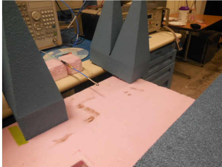
Figure 74. Antenna connected to E5071C network analyzer.
