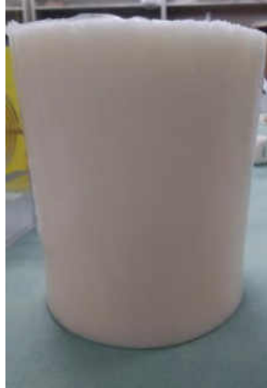
Fig. 7.1. A sample of fabricated tissue phantom.
