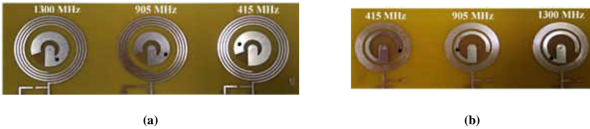
Fig. 7.3. Fabricated combinations of coil/antenna for (a) EX and, (b) IM.
