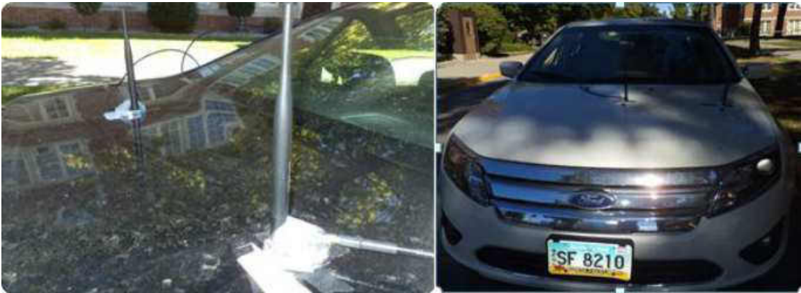
Figure 50: Antennas placement on TX (left) and on RX (right).
