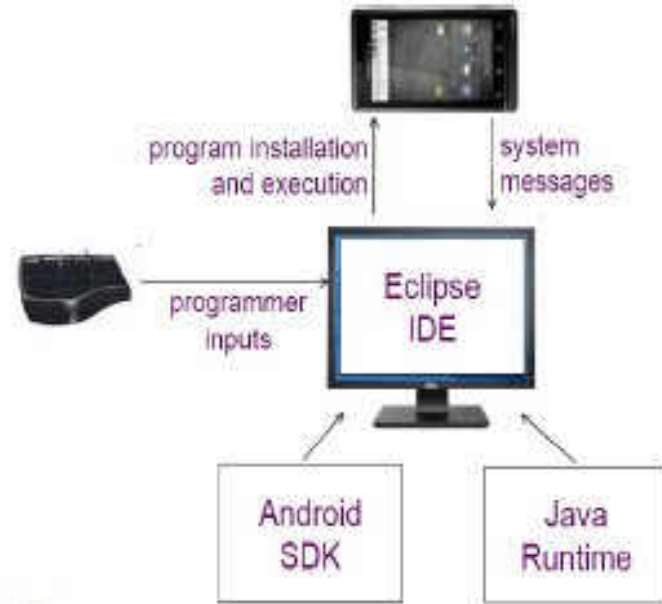
Figure 2. Android Programming Framework. (Gandhewar & Sheikh, 2011, p. 14, reprinted with permission).
