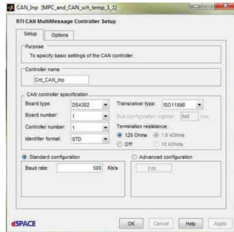
(b) RTI CAN Multi Message controller setup for a sender node.
