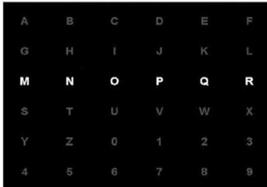
Figure 2.1: The P300 speller interface is displayed as 6 by 6 row-column paradigm (RCP) on the user's screen.
