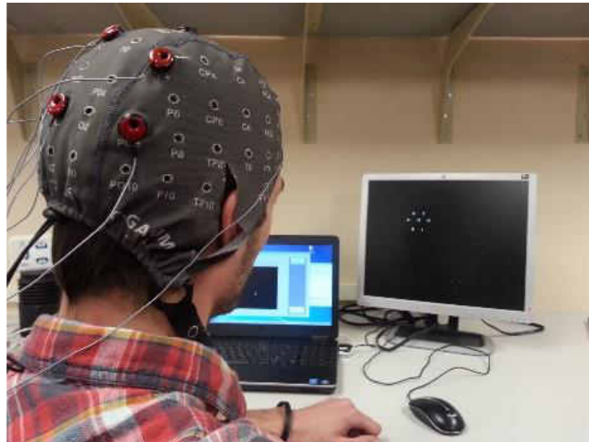
Figure 1.3: EEG data acquisition using a hand-free BCI speller paradigm.
