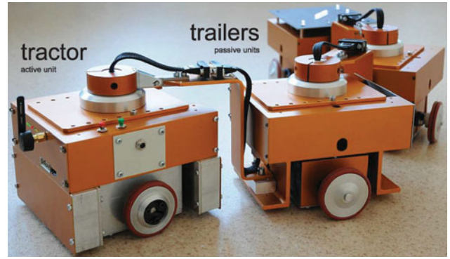
Figure 8. View of the laboratory-scale N-trailer vehicle used in the experiments.
