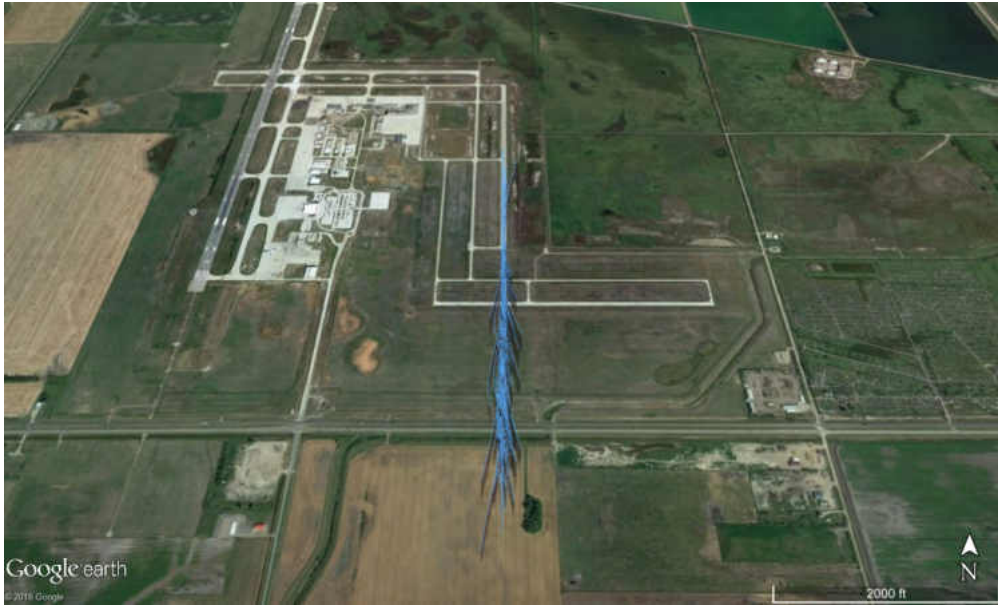
Figure 22: Cluster 1 - Aerial view of the trajectories for the excessively high and fast approaches; 10% of these were aborted.
