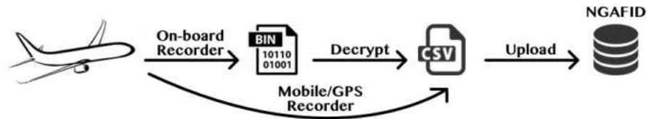
Figure 8: Flight data is recorded using an airborne recording device which may encrypt the data. At the end of each flight the data is manually retrieved from the aircraft, decrypted and converted into a CSV format before it is uploaded to the NGAFID.
