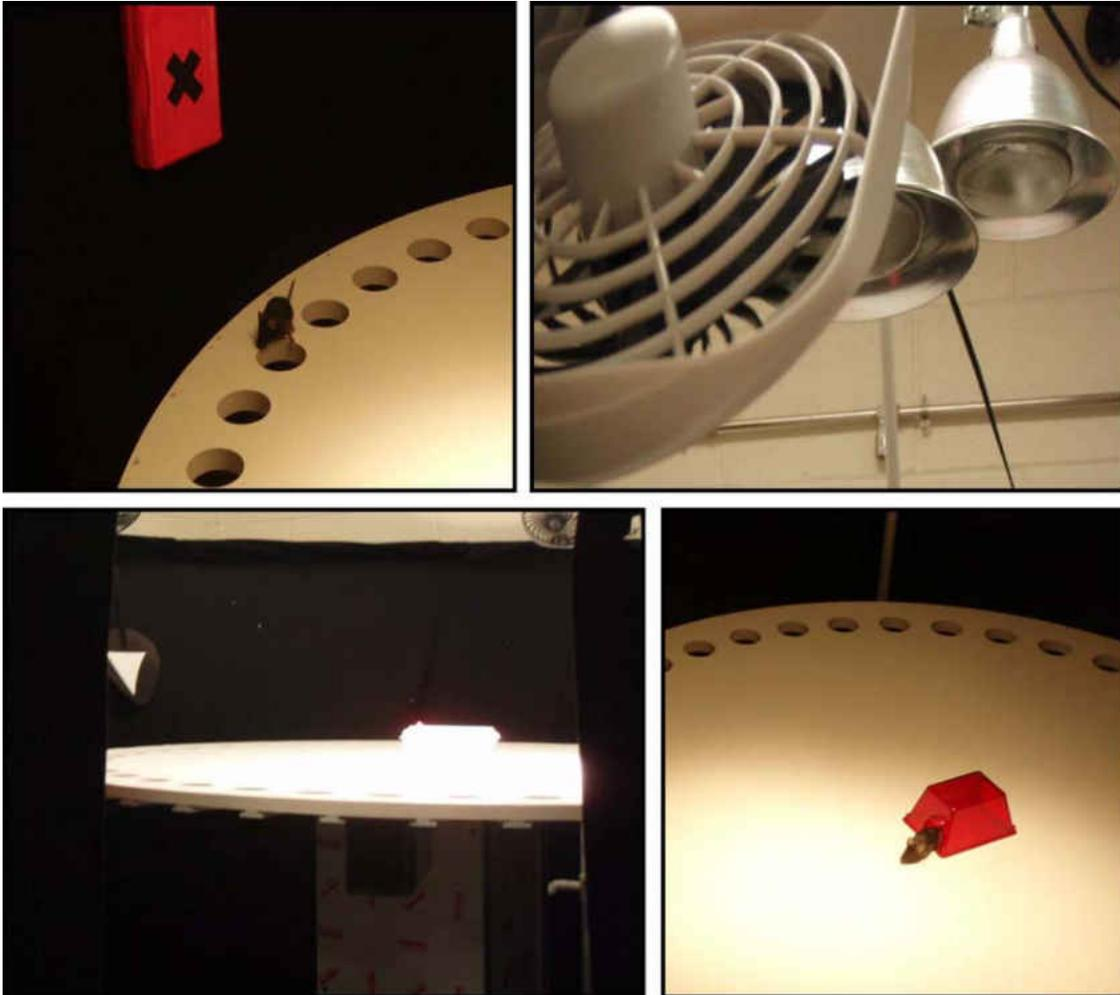
Figure 15. Barnes maze apparatus. (Top left) Mouse navigating the Barnes maze based on spatial cues shown in bright pink and black. (Top right) Aversive stimulus was produced with bright flood lights and fans. (Bottom left) Barnes maze on raised pedestal, showing a large black curtain draped around the apparatus to block distractions. (Bottom right) Mouse in red mouse house moments after being placed on the maze (house will be removed once mouse exits the house).
