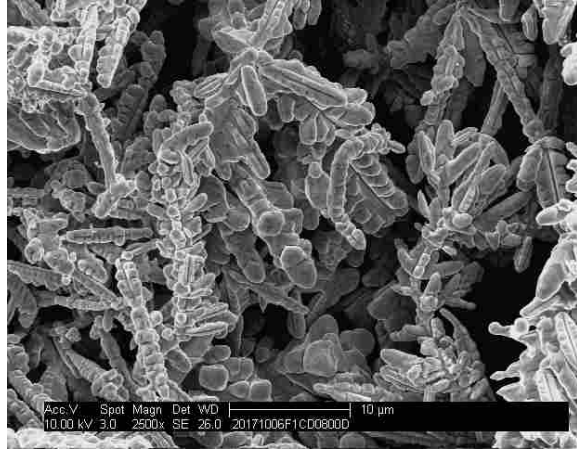
Figure 2-9: SEM image of the dendritic copper powder at 2,500X.
