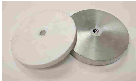
Figure 3-5: Teflon and aluminum impact heads used to test impact material effects.
