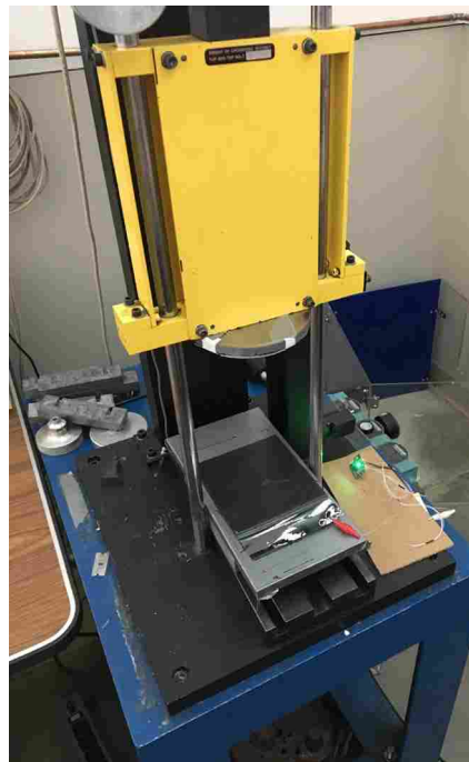
Figure 3-4: Modified Dynatup 8700 impact tester with interchangeable heads.
