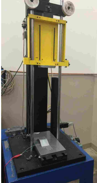
Figure 2-3: Modified Instron drop testing apparatus used in testing NCPF sensors.
