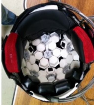
Figure 4-3: Football helmet instrumented with eight NCF sensors which replaced existing helmet padding.
