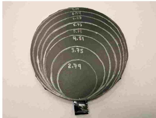
Figure 3-3: NCF sensor used to determine the volumetric effects on response.
