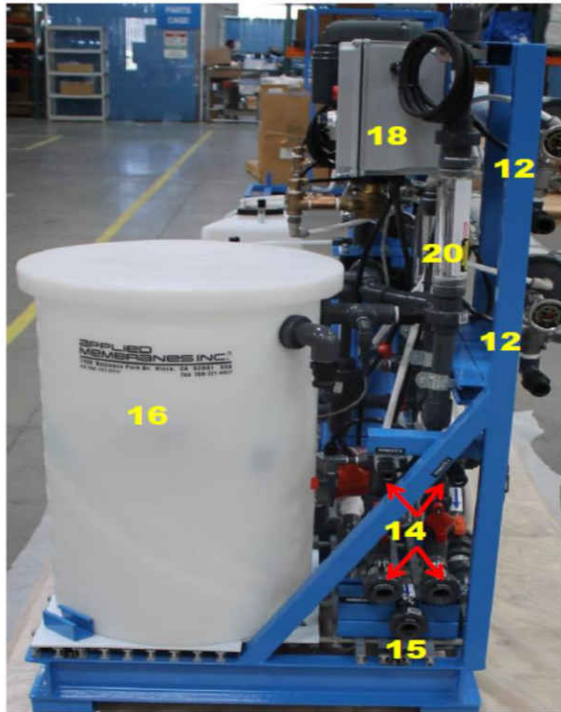
Figure 4.5.4.3. RO pilot system PW-4XM-14A-116 side view.
