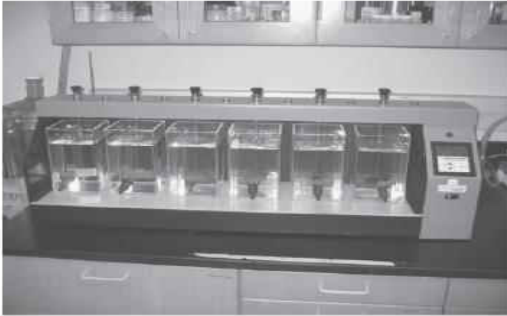
Figure 4.5.2.1. Jar test apparatus. Notably, square containers are used to limit vortex flow formation, wherein particles rotate in the same position relative to each other 89 .
