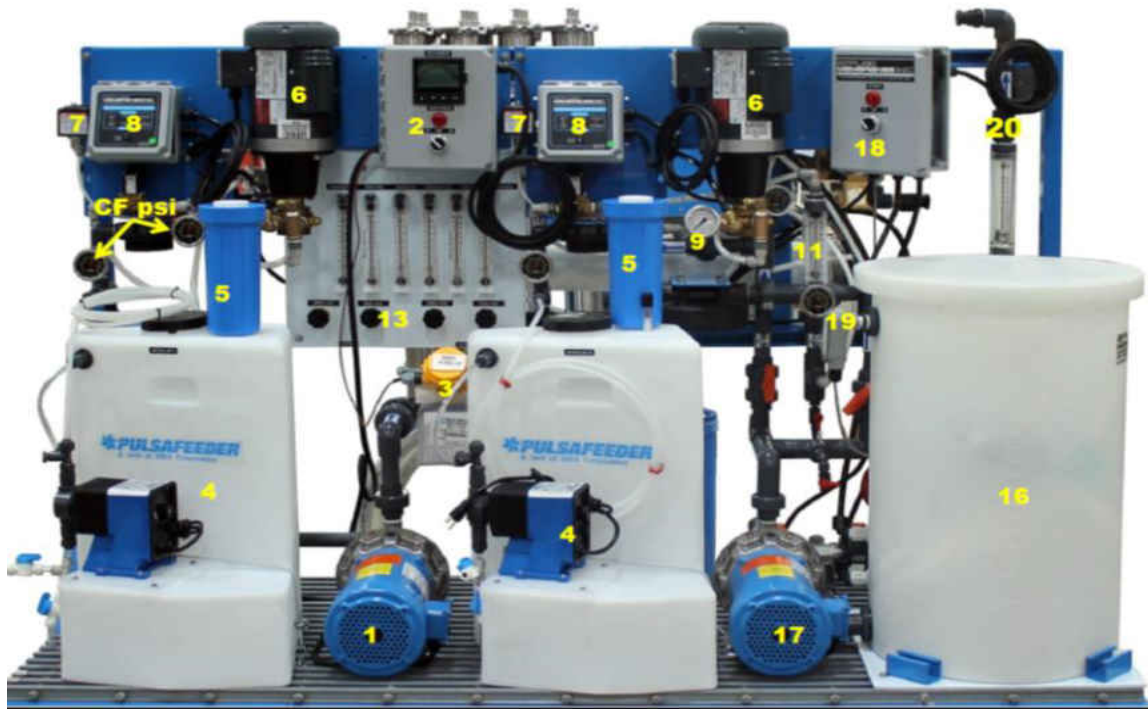
Figure 4.5.4.1. RO pilot system PW-4XM-14A-116 front view.
