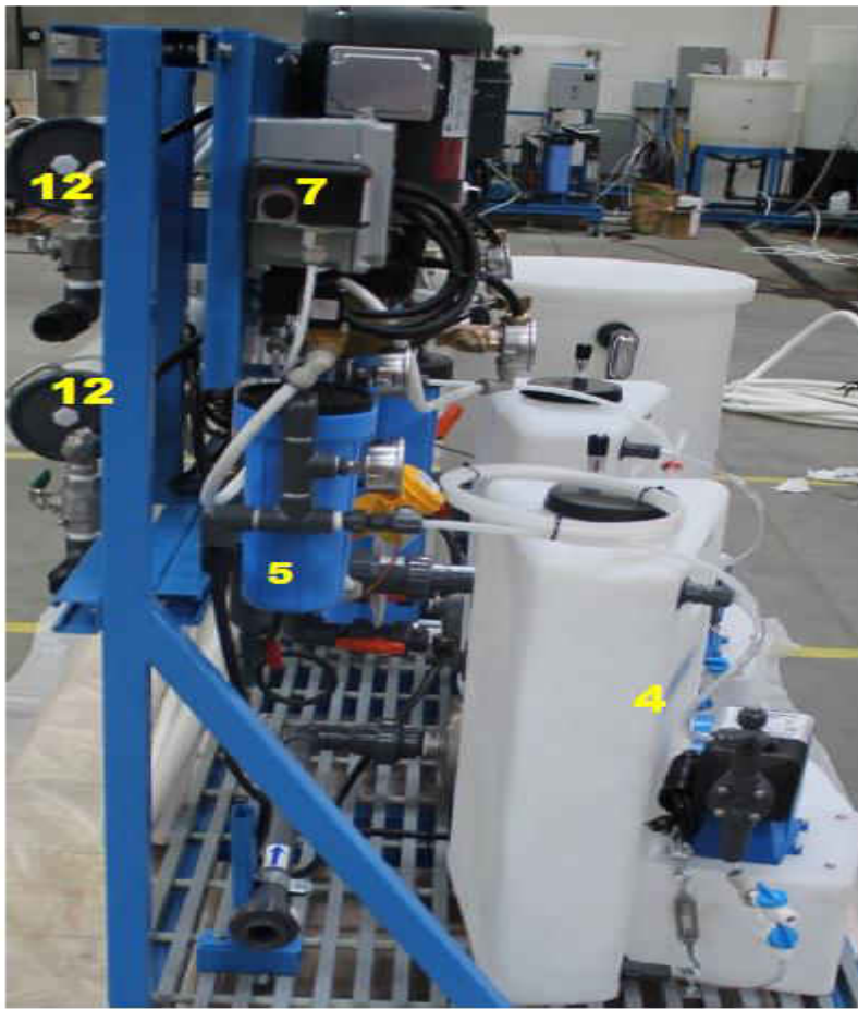
Figure 4.5.4.2. RO pilot system PW-4XM-14A-116 side view.
