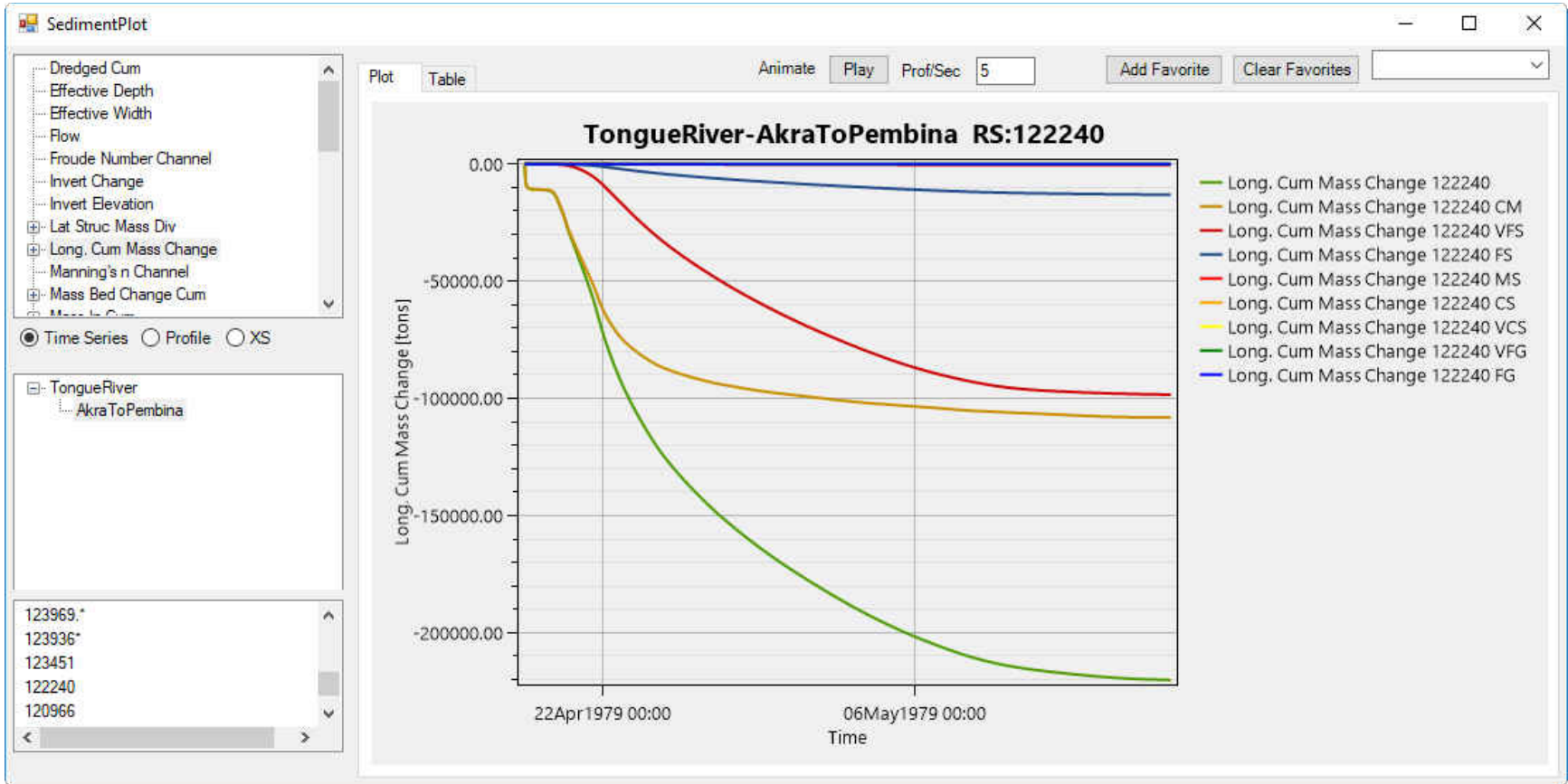
Figure 50. HEC-RAS 100-year sediment cumulative mass change at maximum erosion cross section for Woodland Terrace 5ft weir model
