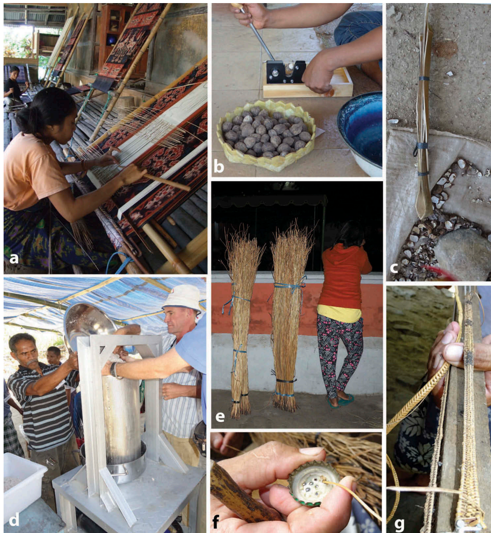
Figure 4. Use of appropriate technologies to add value to natural resource-based enterprises. (a). A loom used to weave traditional textiles. (b). Testing a macadamia nut-cracker developed in Australia for cracking candlenuts (from Aleurites moluccana ). (c). The traditional method of cracking candlenuts, using a tool made from a strip of Areca catechu palm spathe. (d). Using a seed-oil extraction press at a village in West Timor (press built in Java for this project). (e). Stems of the climbing fern Lygodium circinnatum . (f). A bottle top with holes: the local technology to trim fern stems L. circinnatum strips a consistent diameter for a high-quality end product. (g). A wooden frame for weaving complex straps for exported L. circinnatum baskets. Photos: A.B. Cunningham (A–D, F, G) and (h). Cunningham (E).
