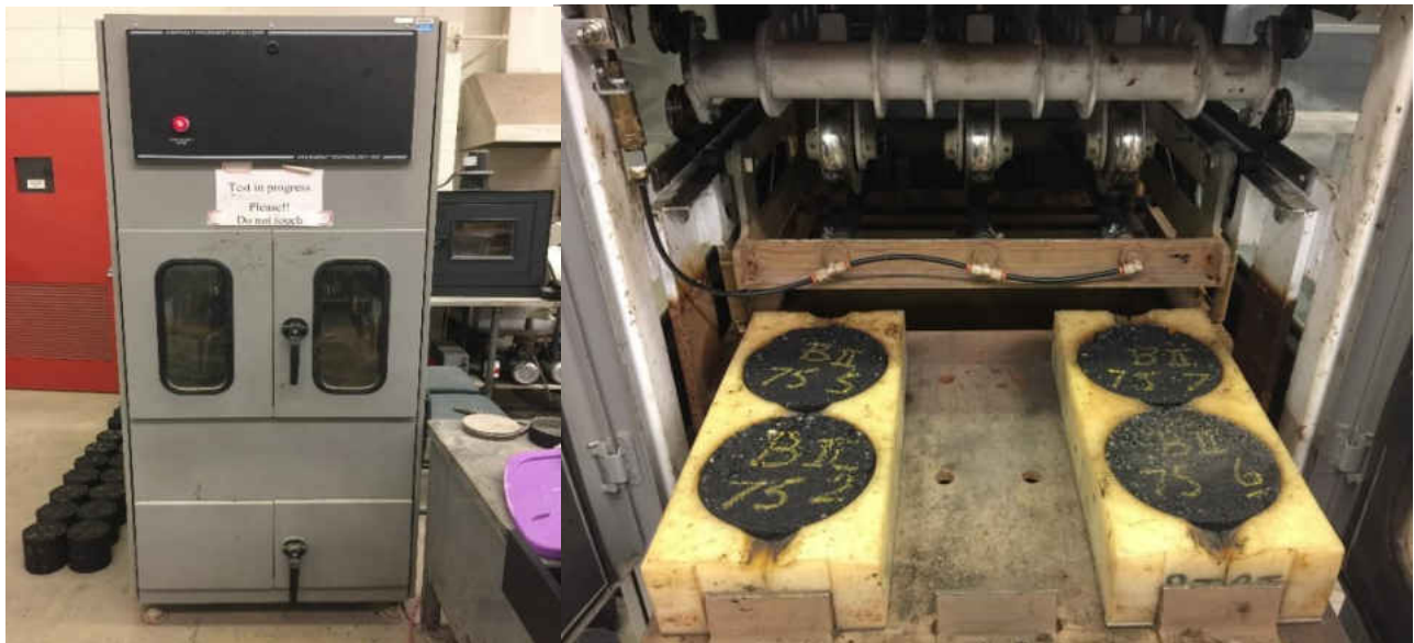
Figure 12. APA Test Setup
