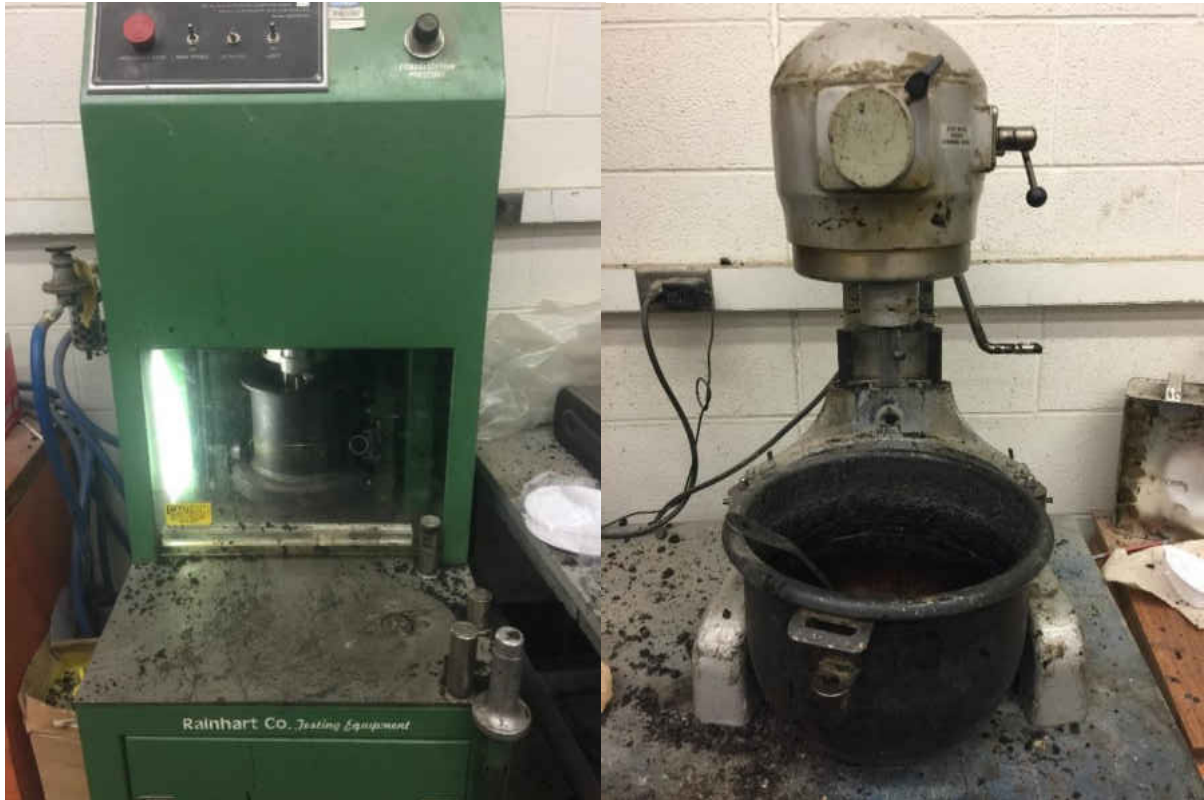
Figure 3. Sample Mixing and Compaction
