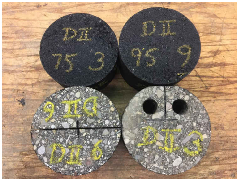
Figure 7. Samples Ready to be Tested
