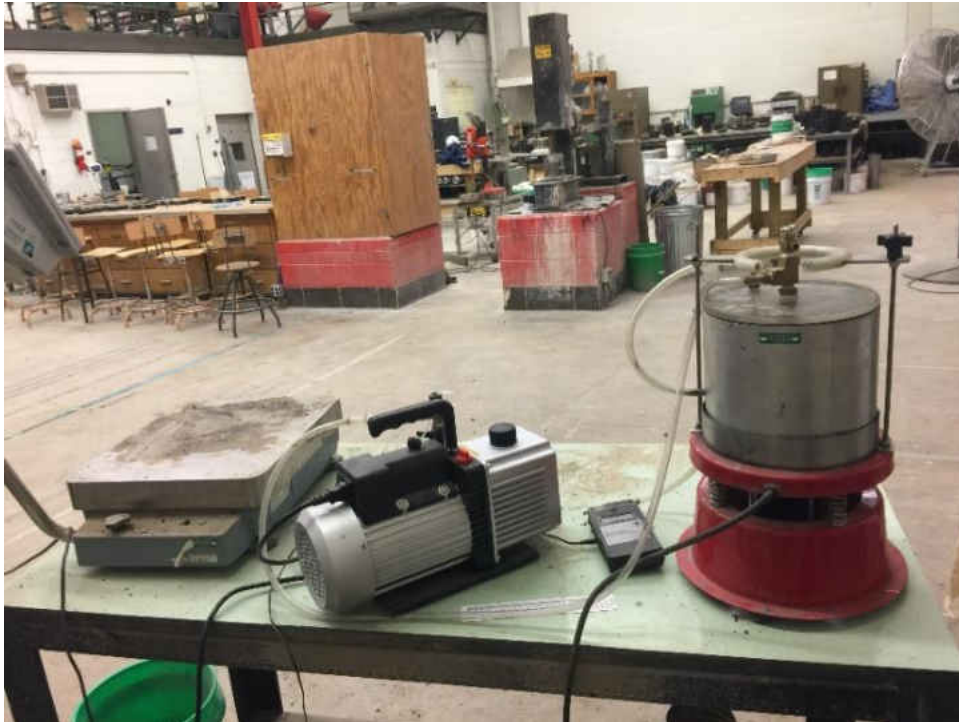
Figure 2. Vacuum Chamber used to determine G_{mm} value
