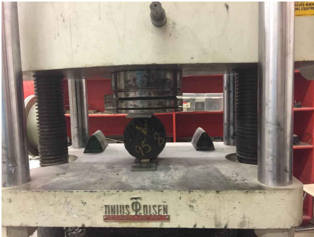
Figure 13. IDT Test Setup
