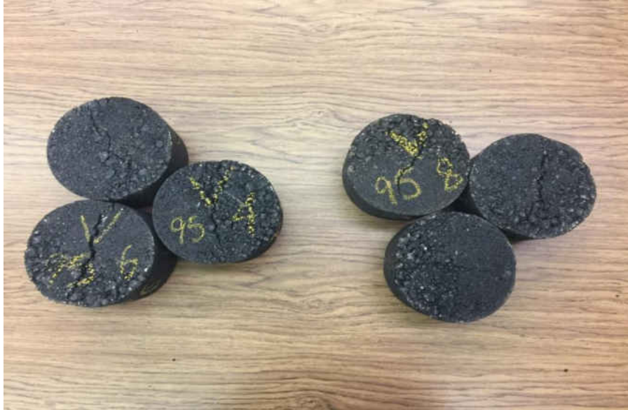
Figure 25. Typical Tested Moisture Damage Specimens
