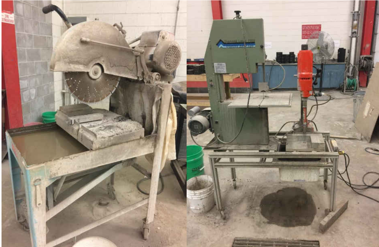
Figure 4. Cutting, drilling and sawing machine
