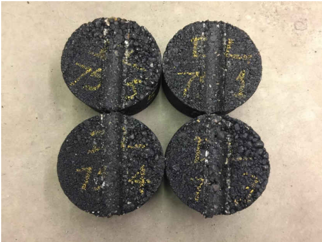
Figure 20. Tested APA Specimens
