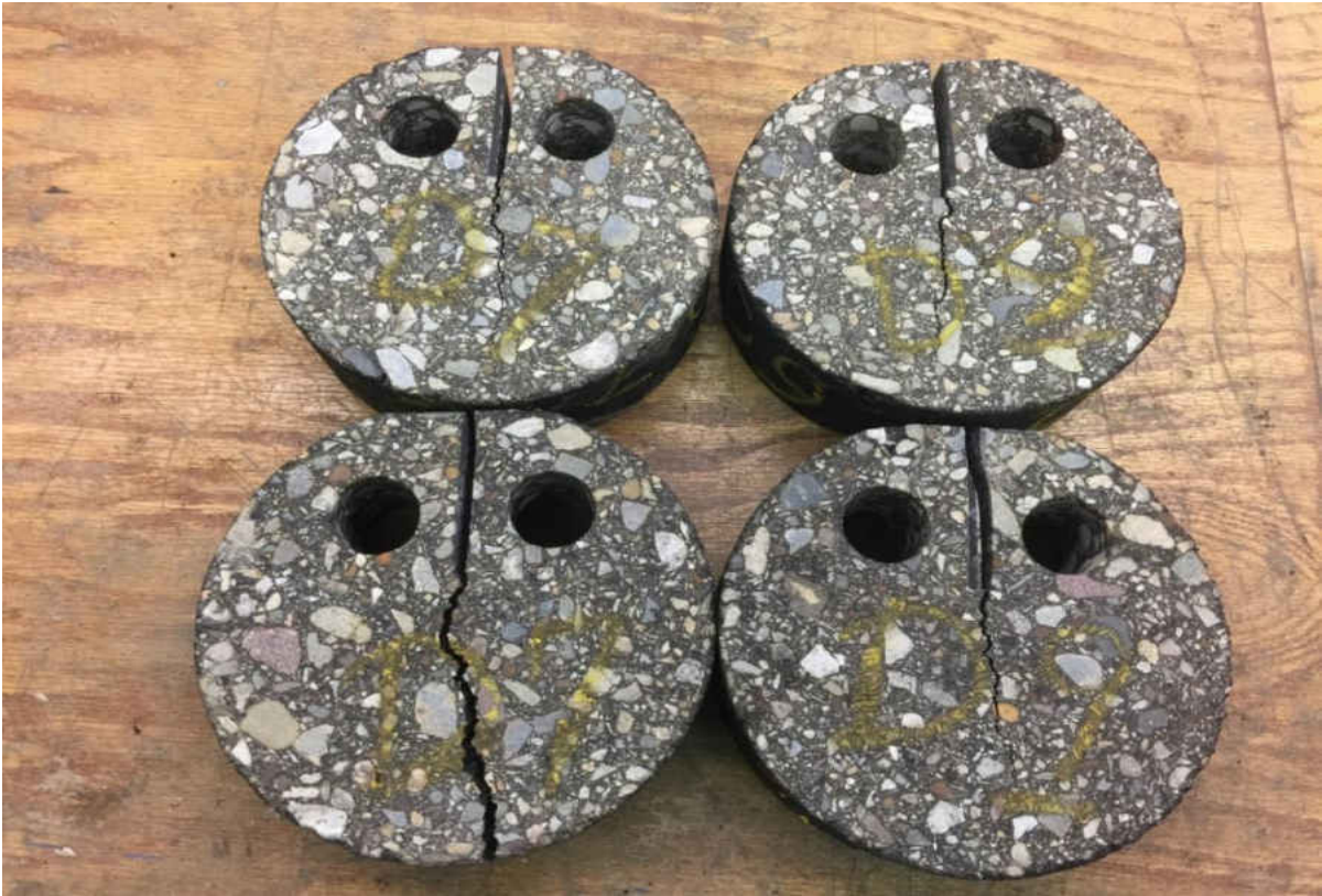
Figure 17. Typical Tested DCT Specimens
