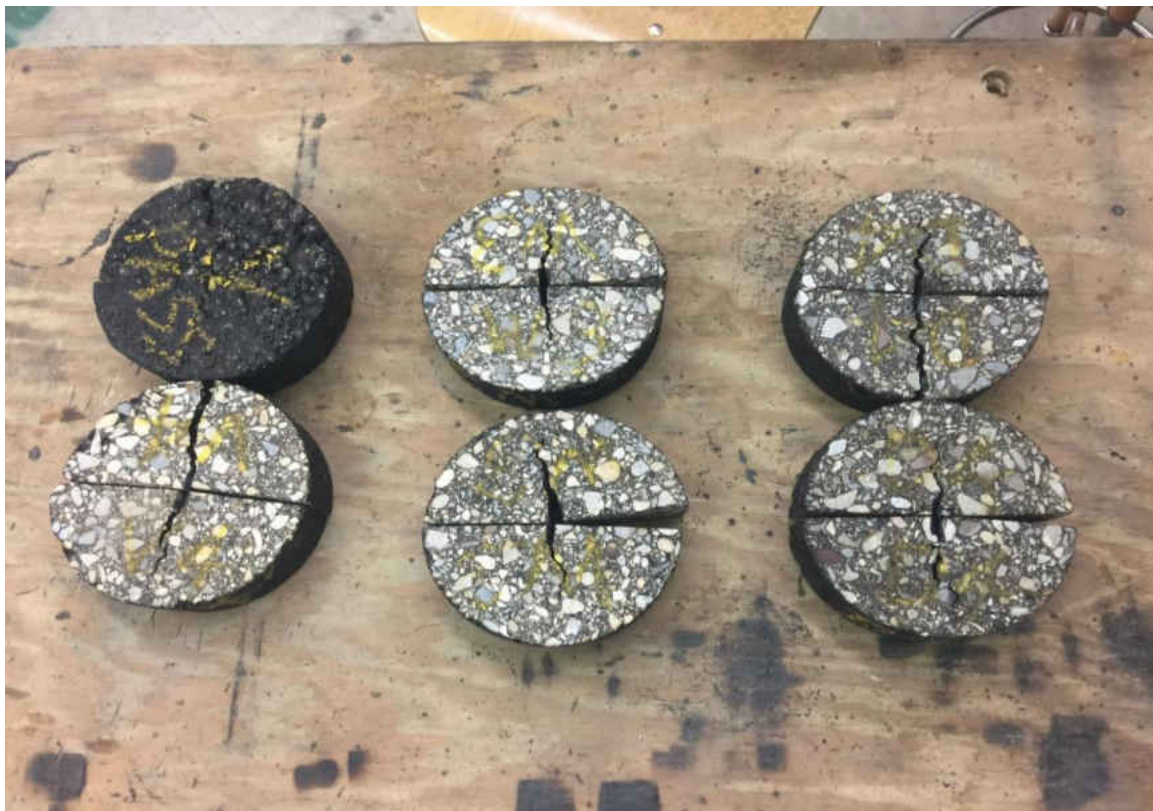
Figure 23. Typical Samples after SCB Tests
