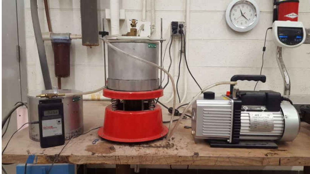
Figure 17. Theoretical Maximum Specific Gravity ( G_{mm} ) Experiment Set-up
