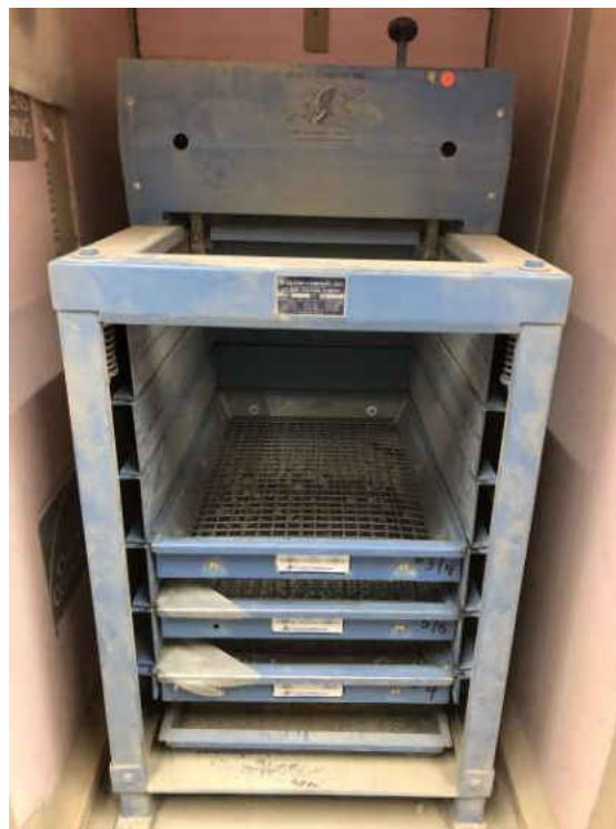
Figure 14. Common set-up of Mechanical Shaker
