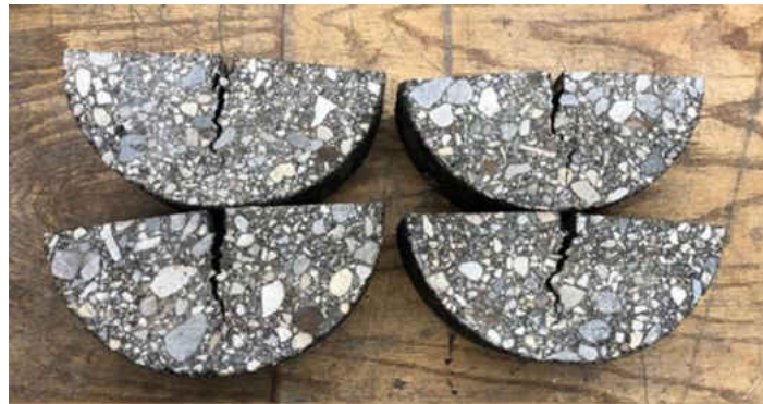
Figure 42. Typical sample after SCB test
