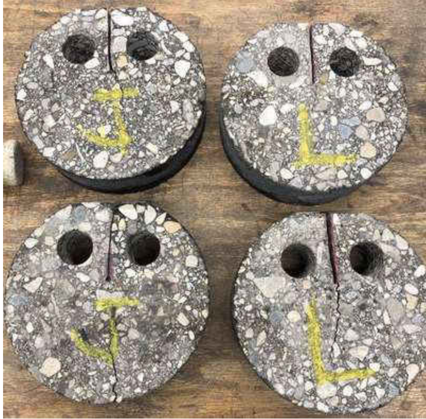
Figure 37. Typical sample after DCT test
