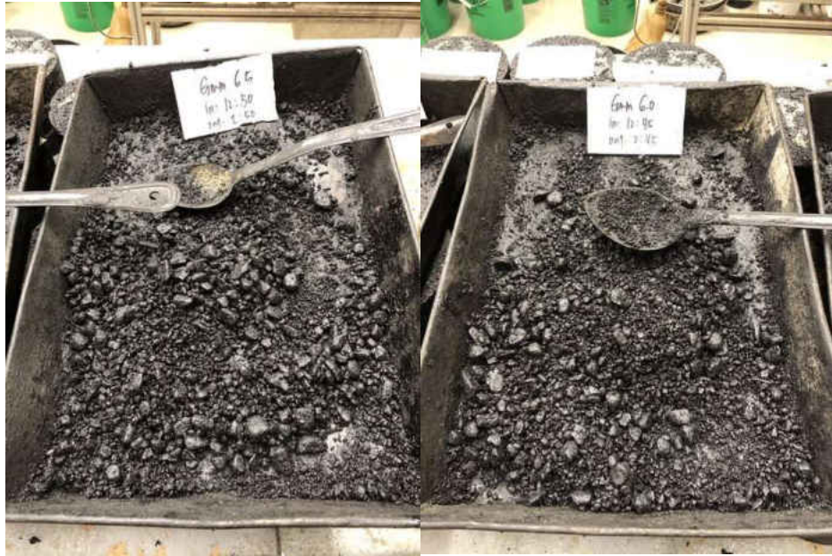
Figure 15. Samples ready for Theoretical Maximum Specific Gravity ( G_{mm} ) testing
