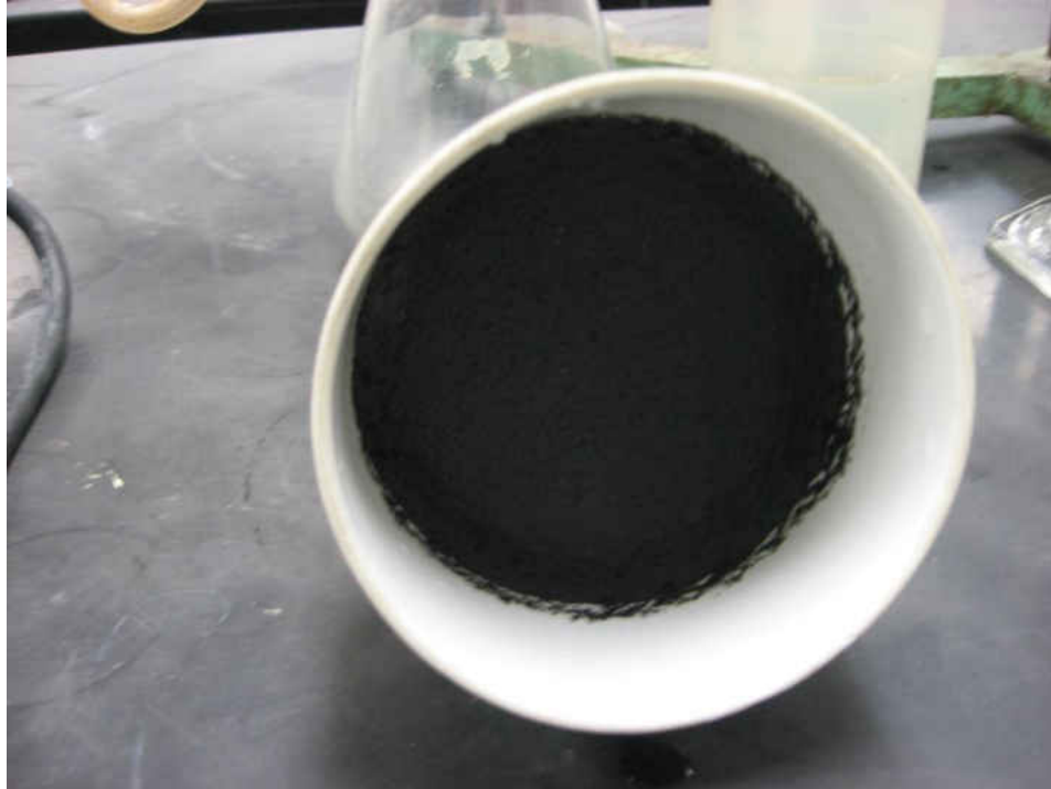
Figure 5.7: Formation of Dry Cake after Applying Vacuum Suction
