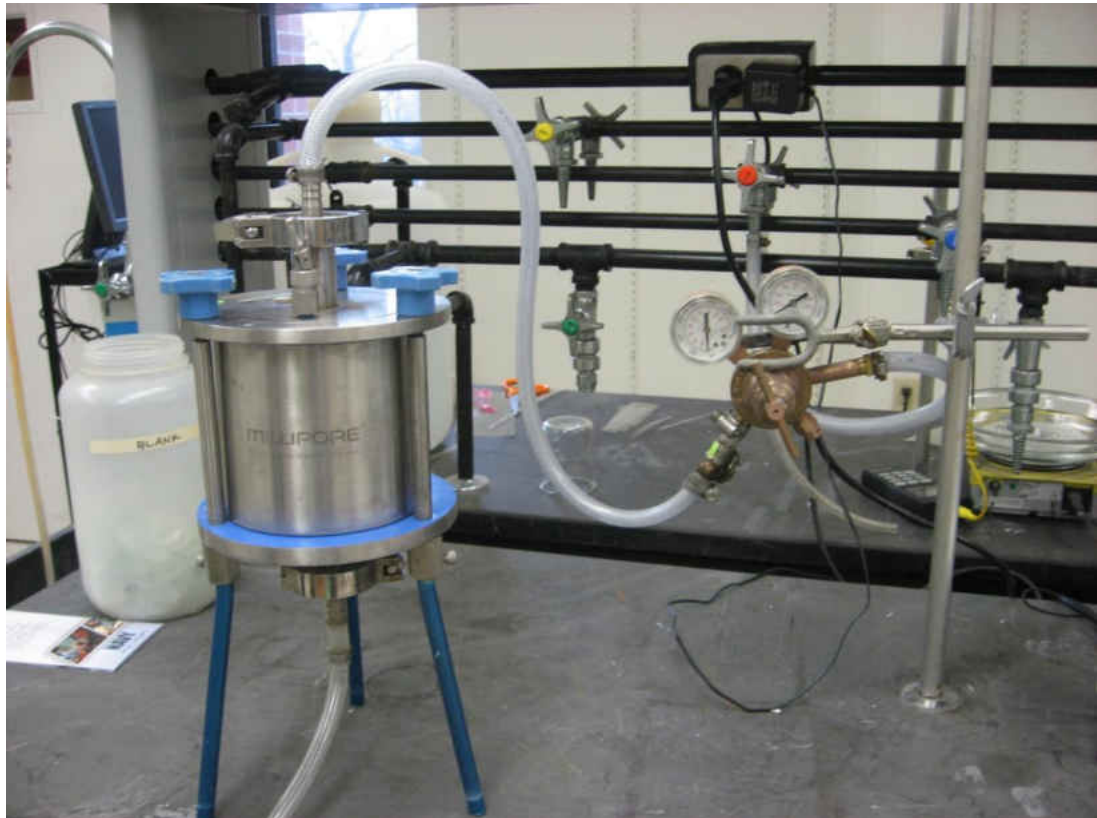
Figure 5.8: Apparatus Assembly for Air Pressure Filtration Test
