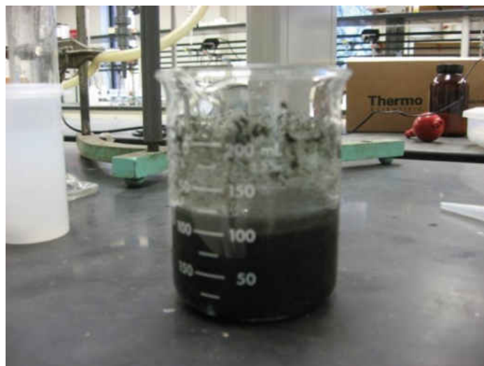
Figure 5.6: Sludge Sample after Mixing with Polymer
