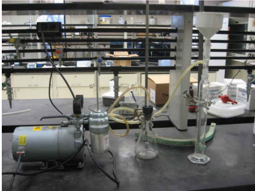
Figure 5.4: Apparatus Assembly for Time to Filter Test
