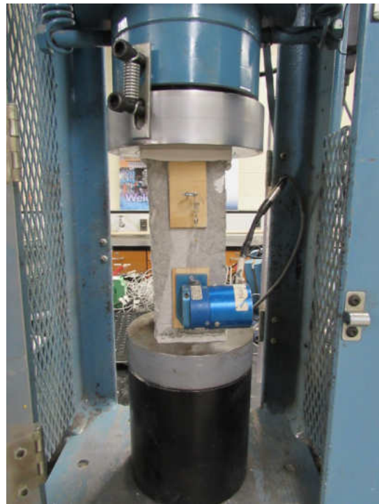
Figure B-2: Testing of Grout Prism Sample using a String Pot
