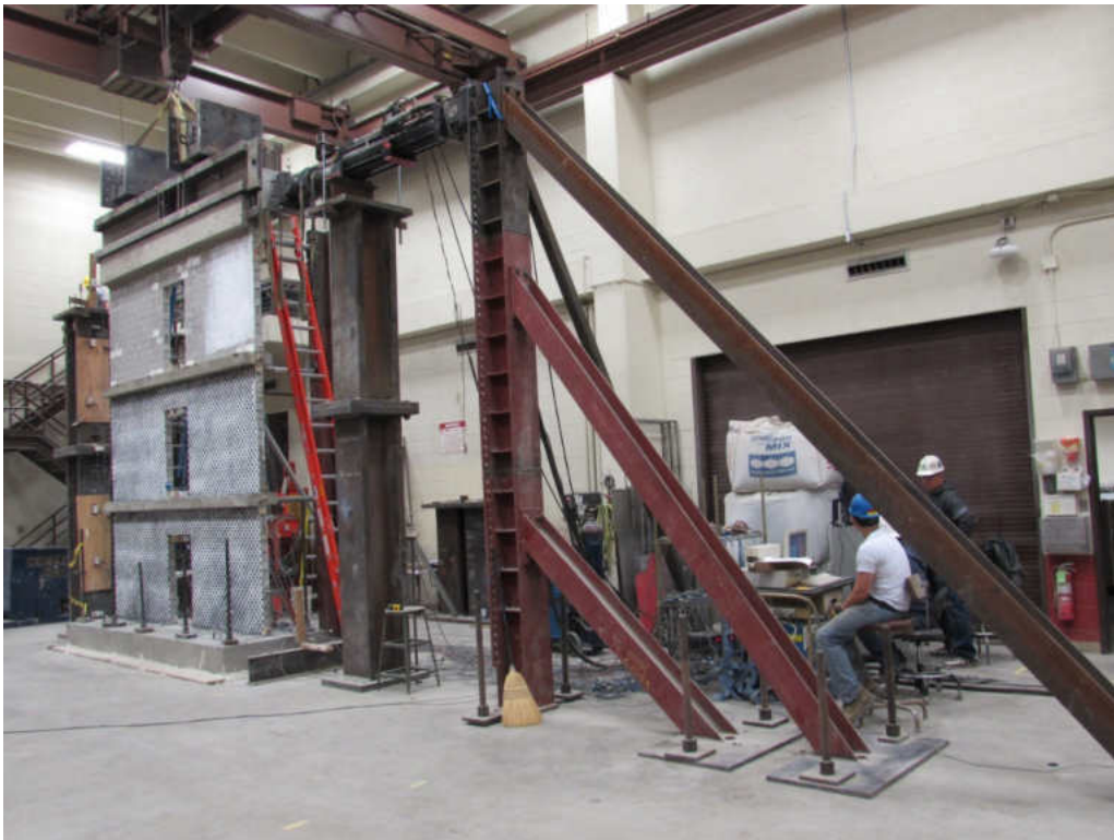
Figure 3-6: Wall Testing Apparatus
