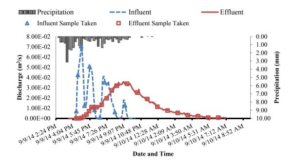
Figure 6. Influent and effluent hydrographs and precipitation hydrograph for 09/09/14 sampling event.
