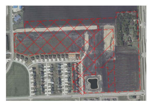
Figure 2. Drainage area delineation.
