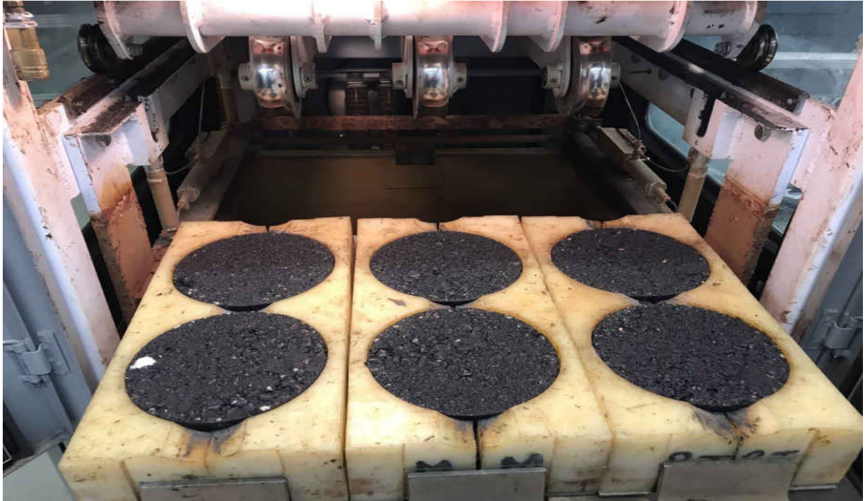
Figure 4.8. APA specimen layout before test
