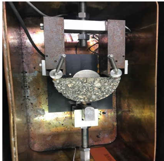
Figure 3.8. SCB before test
