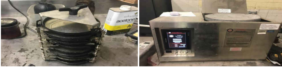
Figure 3.2. Pressure aging vessel (PAV) test assembly
