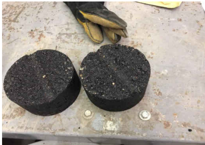
Figure 3.6. AASHTO TP63 test specimen
