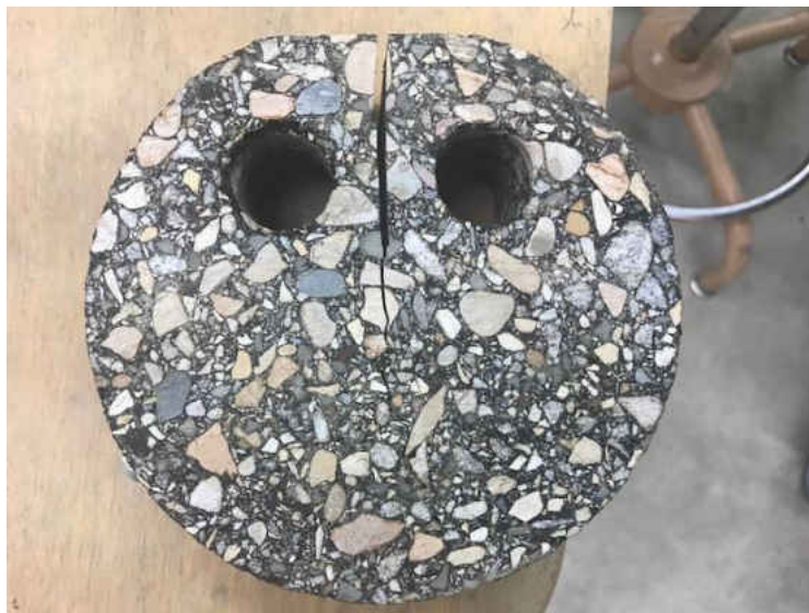
Figure 4.16. Example of DCT specimen after the test
