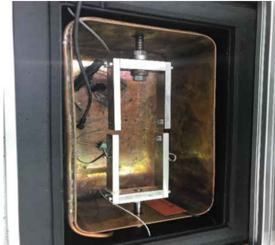
Figure 3.7. DCT test assembly
