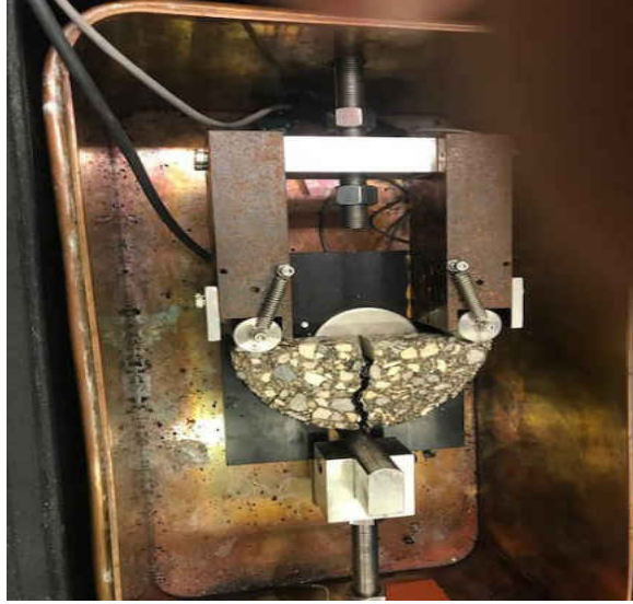
Figure 3.9. SCB after test
