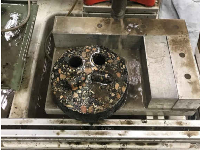
Figure 4.15. Example of DCT specimen prior to test
