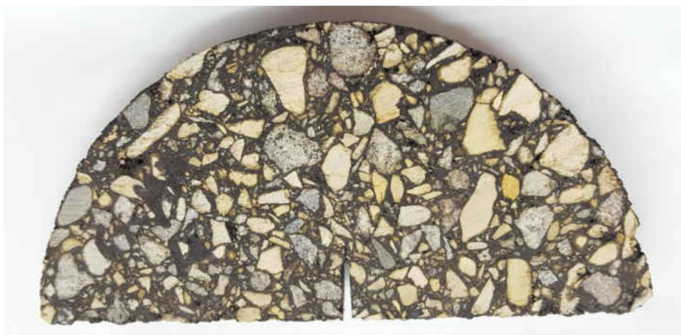
Figure 69. Example of SCB Specimen Prior to Test
