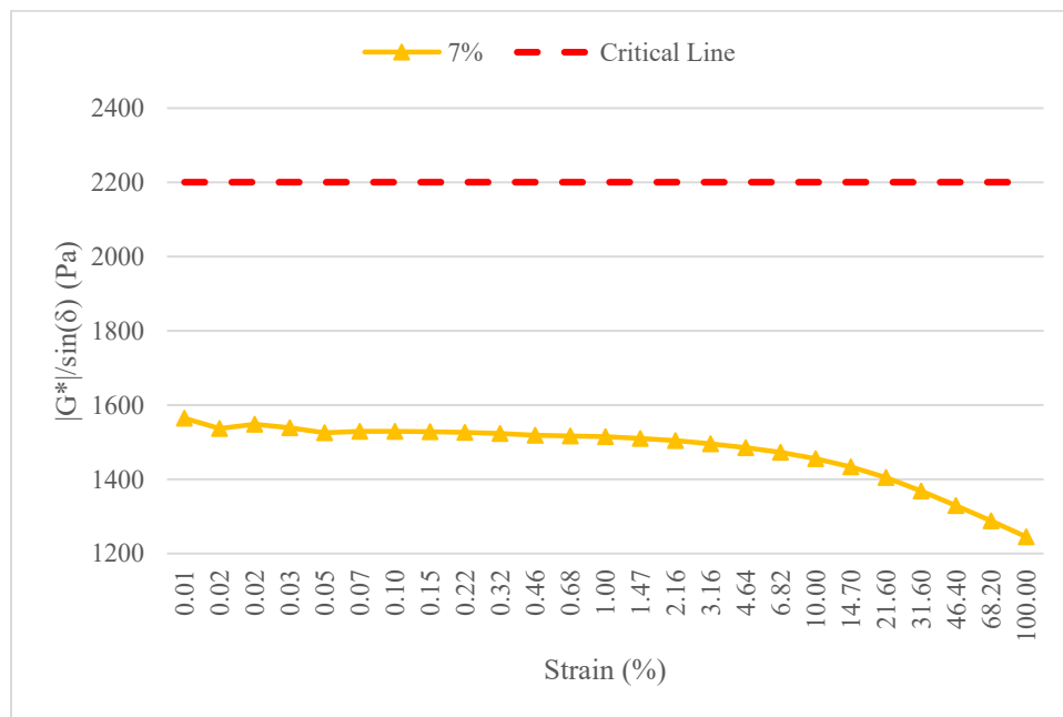
Figure 28. RTFO-aged PG 58-28 modified with 7% NC at 70°C
