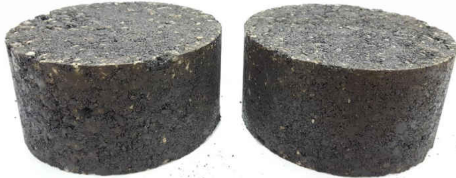
Figure 60. Example of APA Specimen Prior to Test
