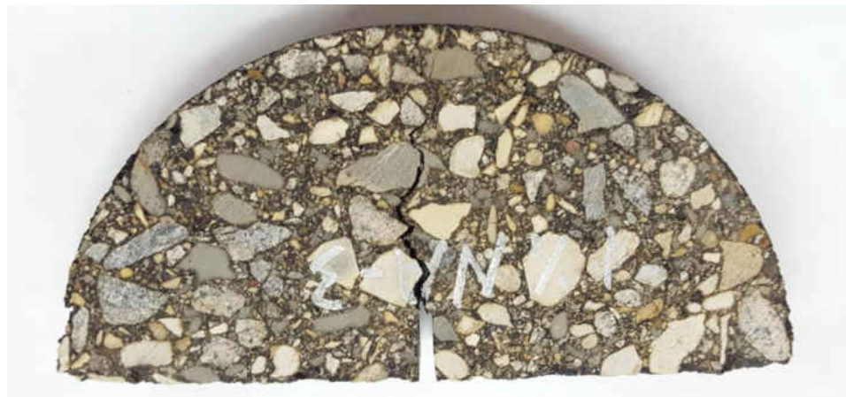
Figure 70. Example of SCB Specimen Post-Testing
