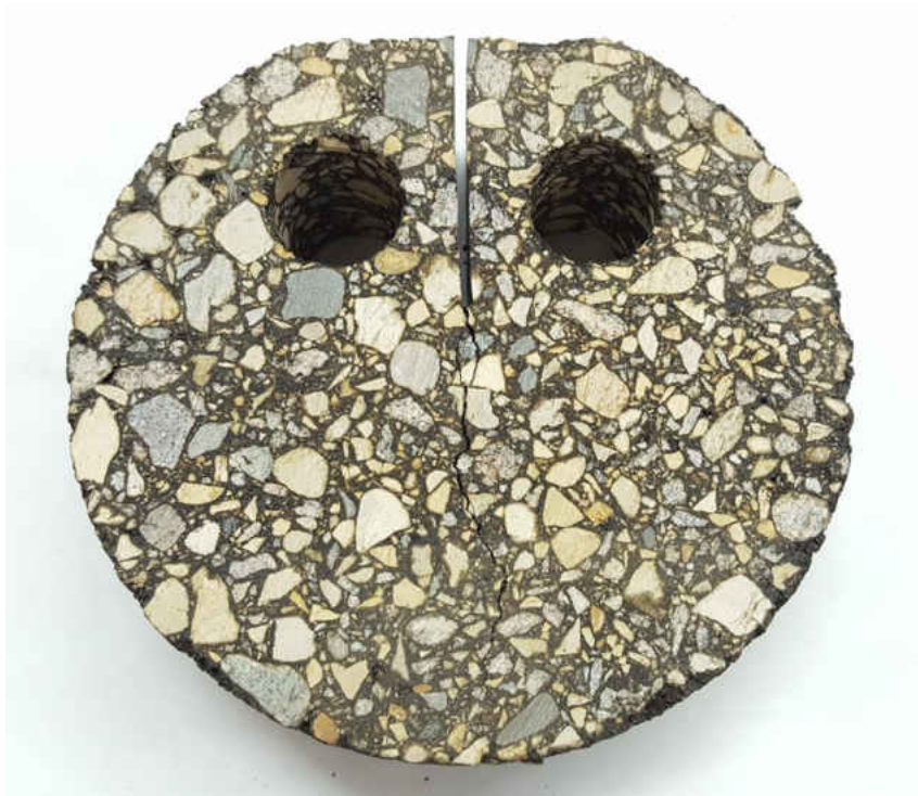
Figure 75. Example of DCT Specimen Post-Testing
