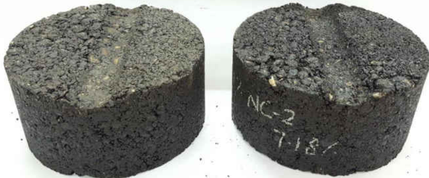
Figure 61. Example of APA Specimen Post-Testing
