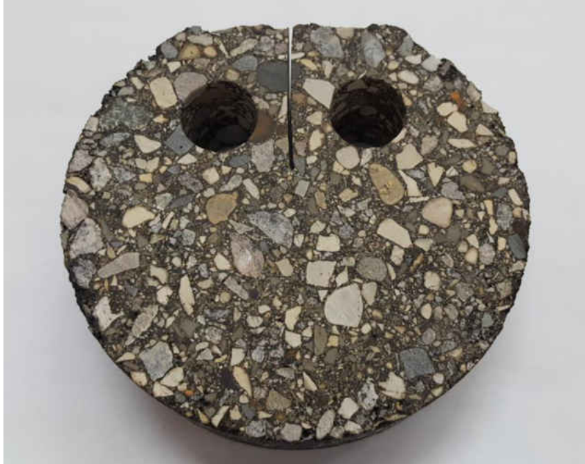
Figure 74. Example of DCT Specimen Prior to Test
