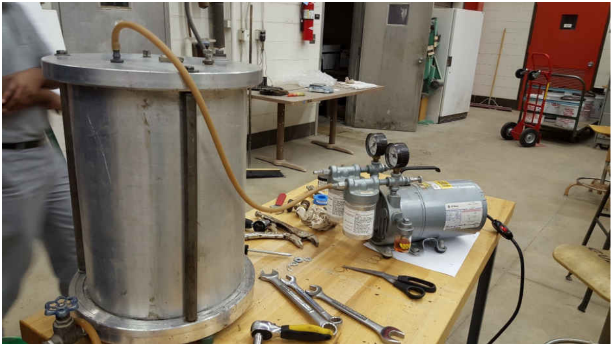
Figure 5 Wet test specimen subjected to vacuum saturation.
