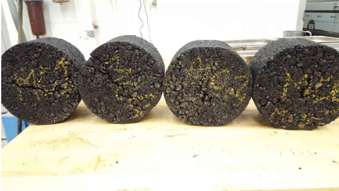
Figure 16 Visible Cracking in the wet Conventional specimens after Modified Lottman Test
