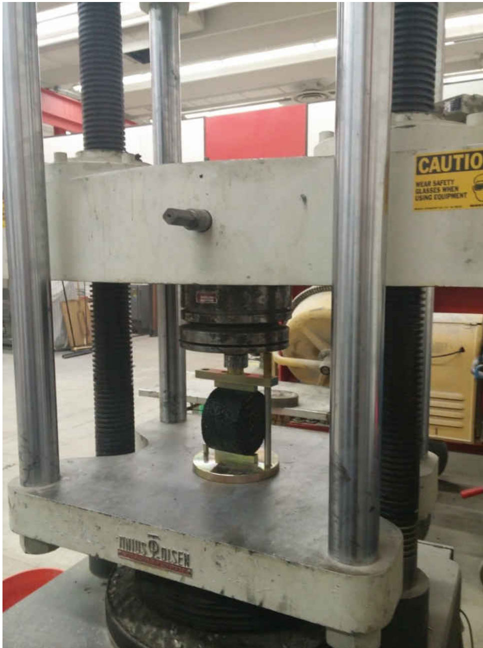
Figure 6 Specimen placement between bearing plates
