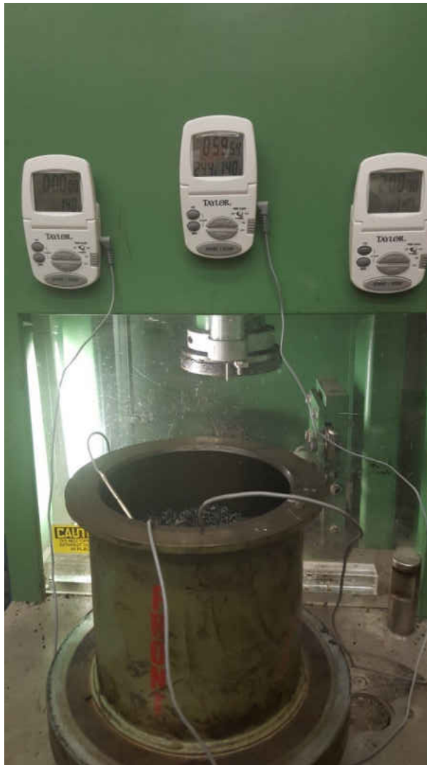
Figure 7 Using 3 thermometers to ascertain even temperature before compaction.
