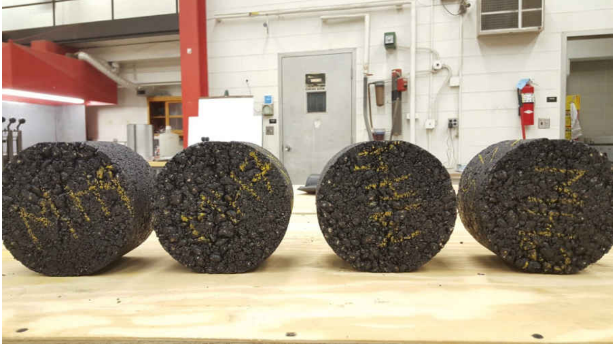
Figure 15 Visible Cracking in the dry Non-Conventional specimens after Modified Lottman Test
