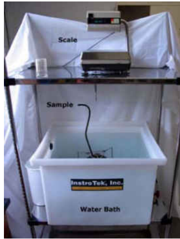
Figure 3.2. Submerging sample for 4 minutes and recording submerged mass
