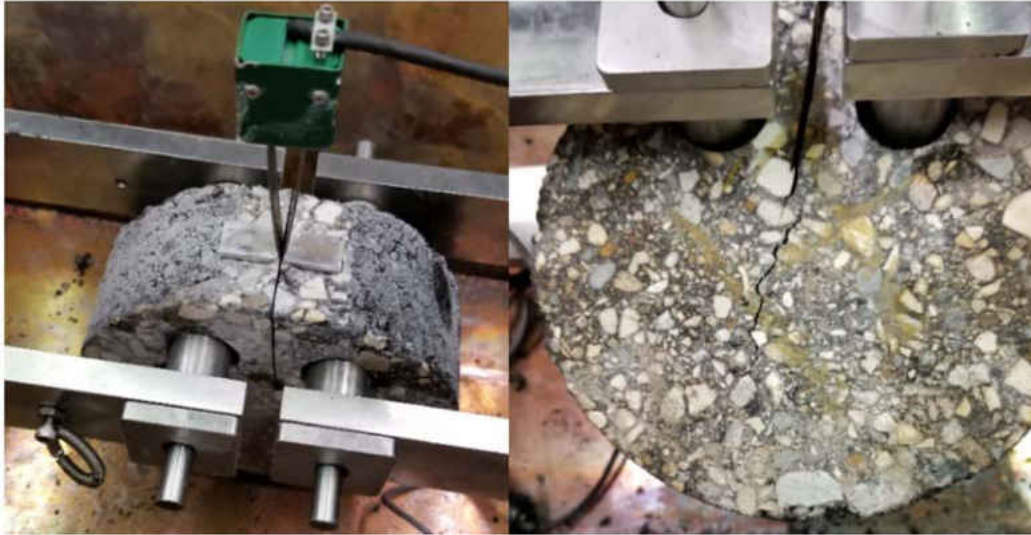
Figure 4.3. DCT Sample: (a) Ready for Testing (left), (b) Test Completed (right)
