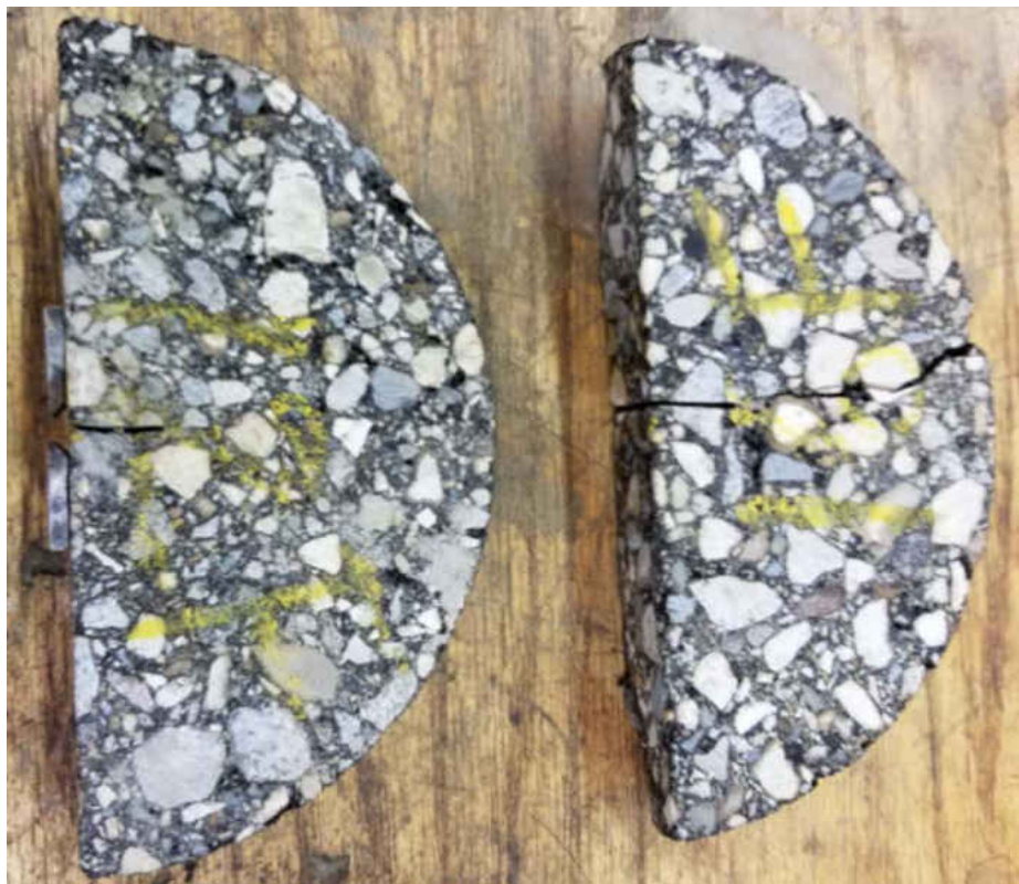
Figure 4.10. SCB Sample: (a) Ready for Testing (left), (b) Test Completed (right)
