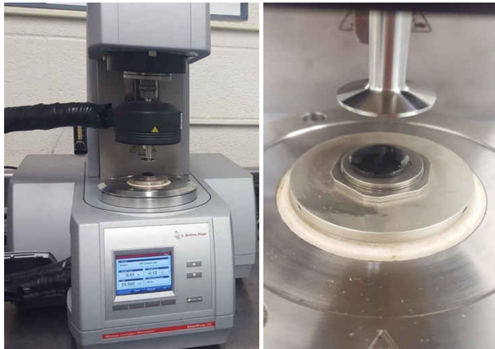
Figure 7: DSR test setup.
