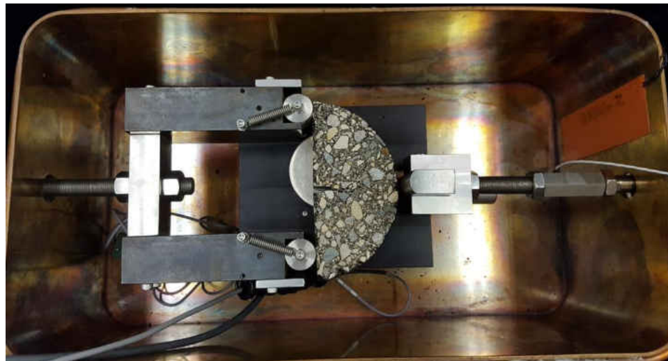
Figure 16: SCB test setup.
