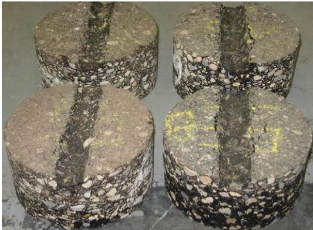
Figure 4: Rut depth by using APA: HMA, left, and WMA on the right
