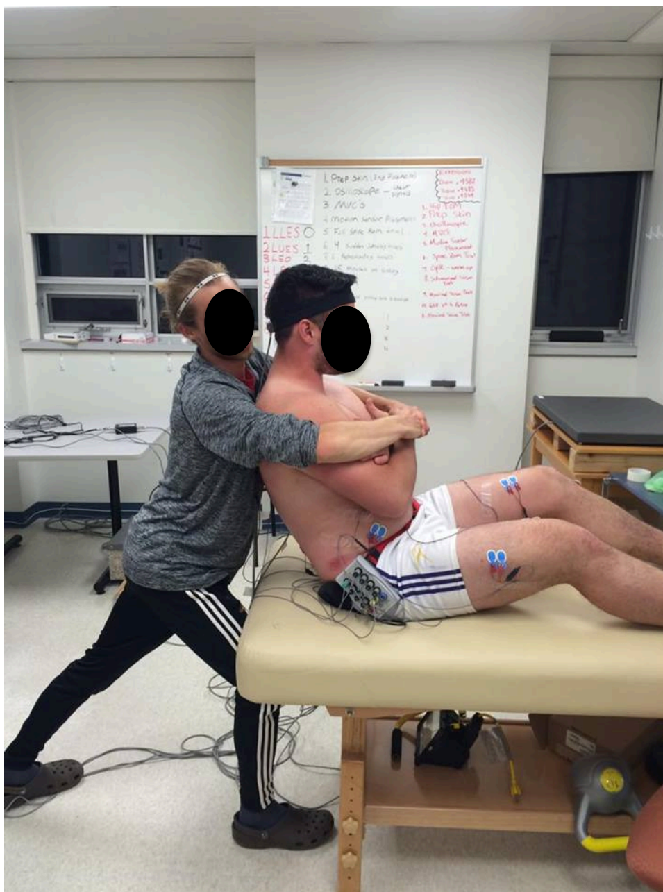
Figure D3. Abdominal MVC. Participant would perform a resisted sit-up, axial twists and lateral bends.
