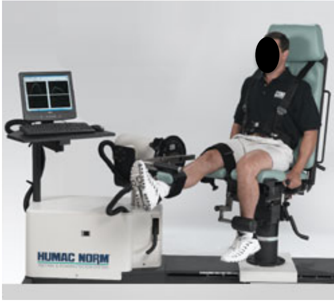
Figure A1. Quadriceps Extension on the Cybex dynamometer. Retrieved from: http://www.isokinetic.info/
