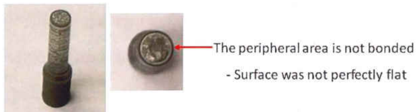
Figure 12. Fracture surface of tensile specimen, faying surfaces were polished by hand before bonding.
