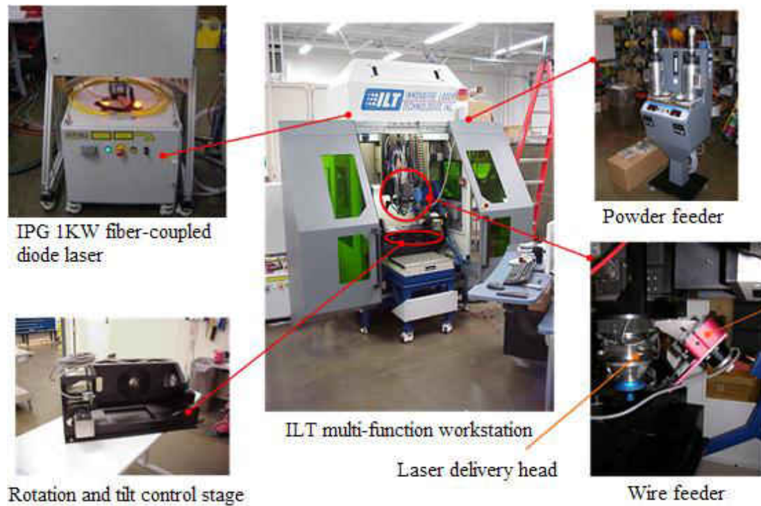
Figure 9. Fiber coupled diode laser system and peripherals at the University of North Dakota's Advanced Engineered Materials Center
