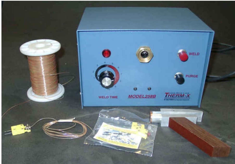
Figure 39. Thermocouple welder, materials, and completed thermocouple.
