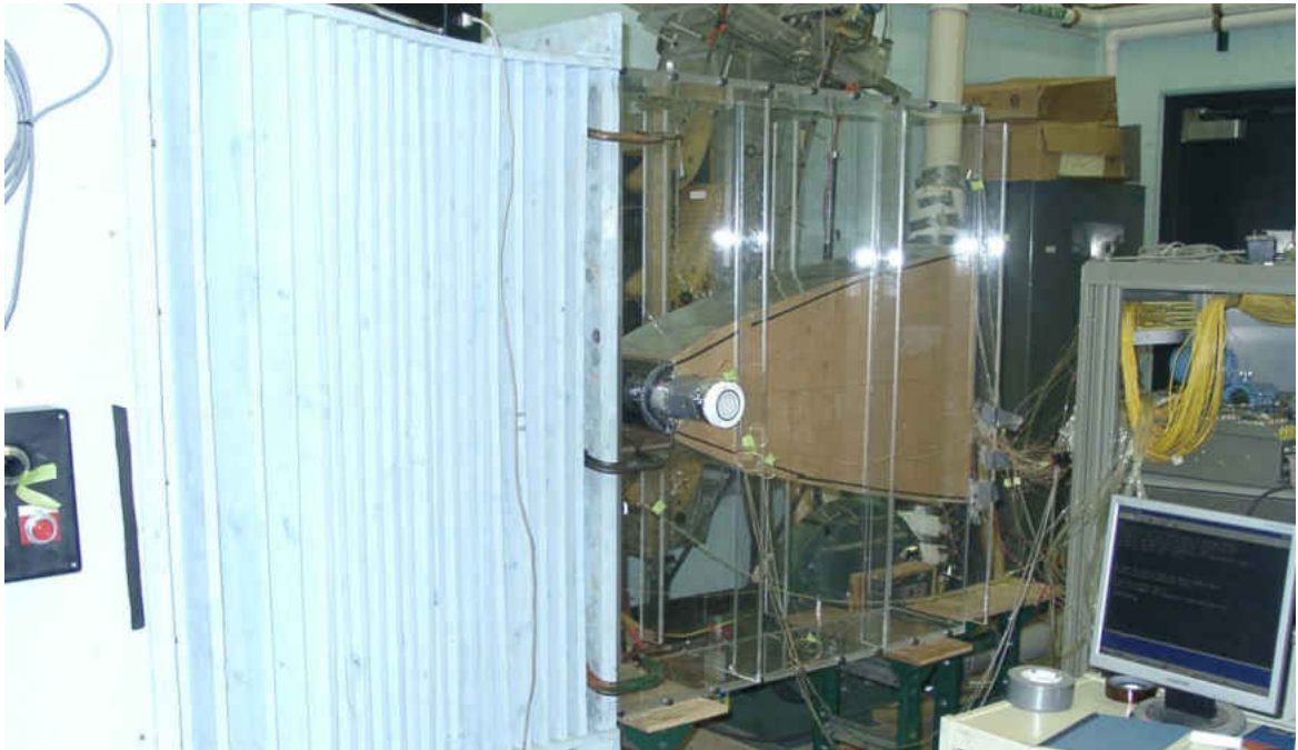
Figure 43. Small cylindrical leading edge test section at low turbulence, no blowing.
