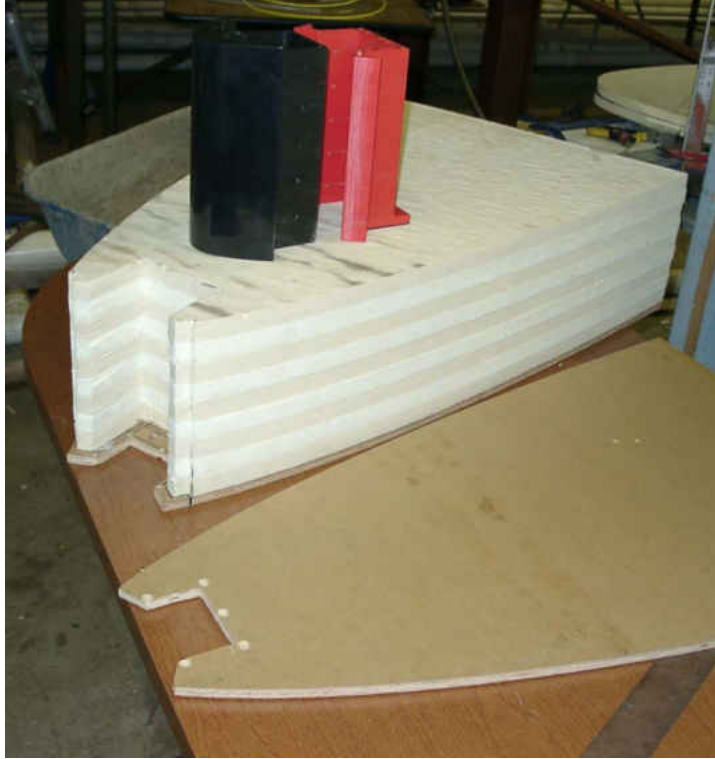
Figure 34. Glued, cut, and drilled small test section with leading edge and mounting bracket.
