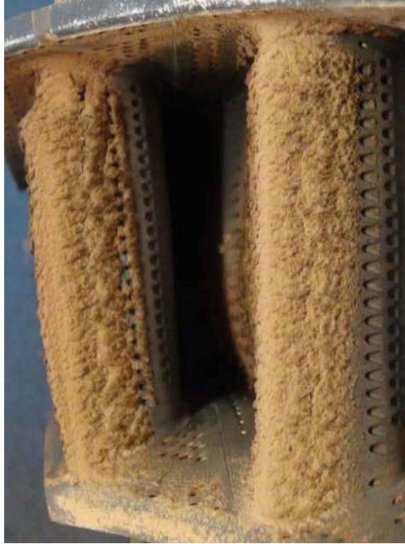
Figure 2. Turbine vane without film cooling [2].
