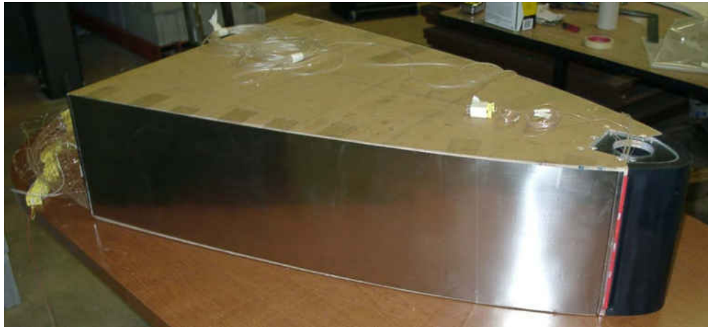
Figure 38. Small cylindrical test section with inconel foil and acrylic window attached.
