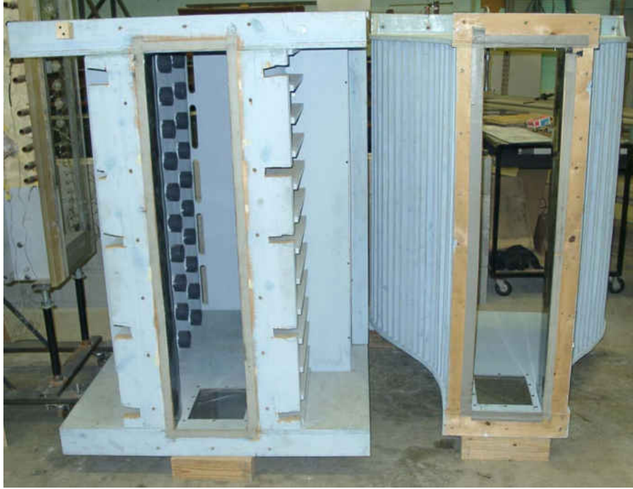
Figure 14. Mock aero-combustor and laminar flow nozzle, front view.
