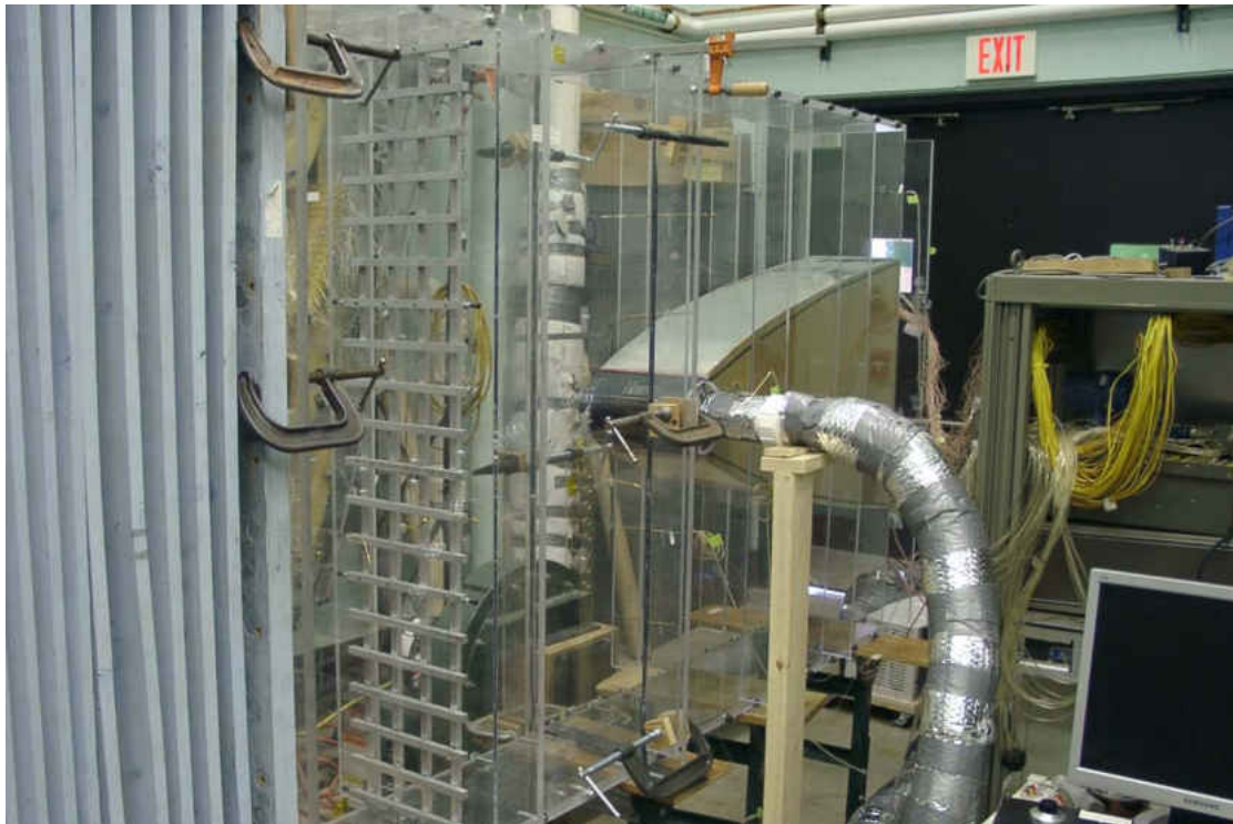
Figure 46. Small cylindrical test section, large grid.
