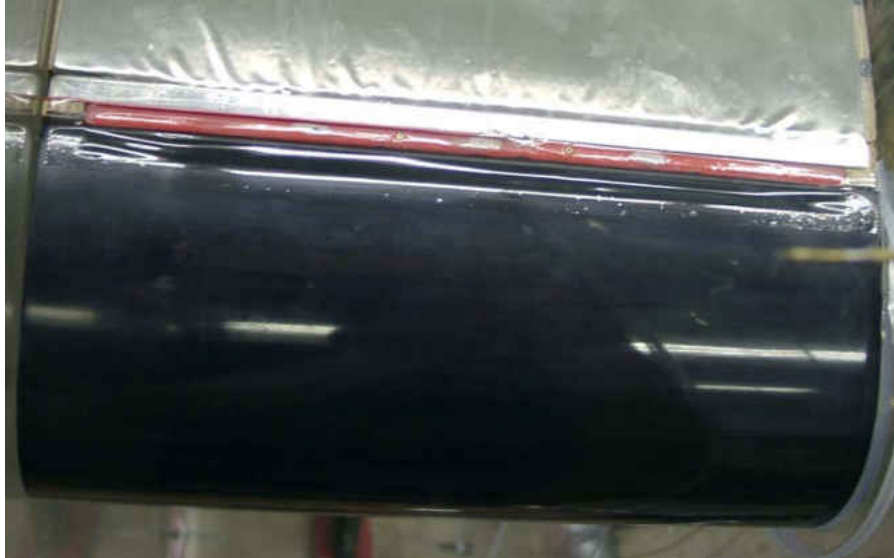
Figure 42. Small cylindrical leading edge test section with slot taped.
