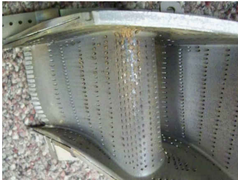
Figure 1. Turbine Vane with film cooling [2].
