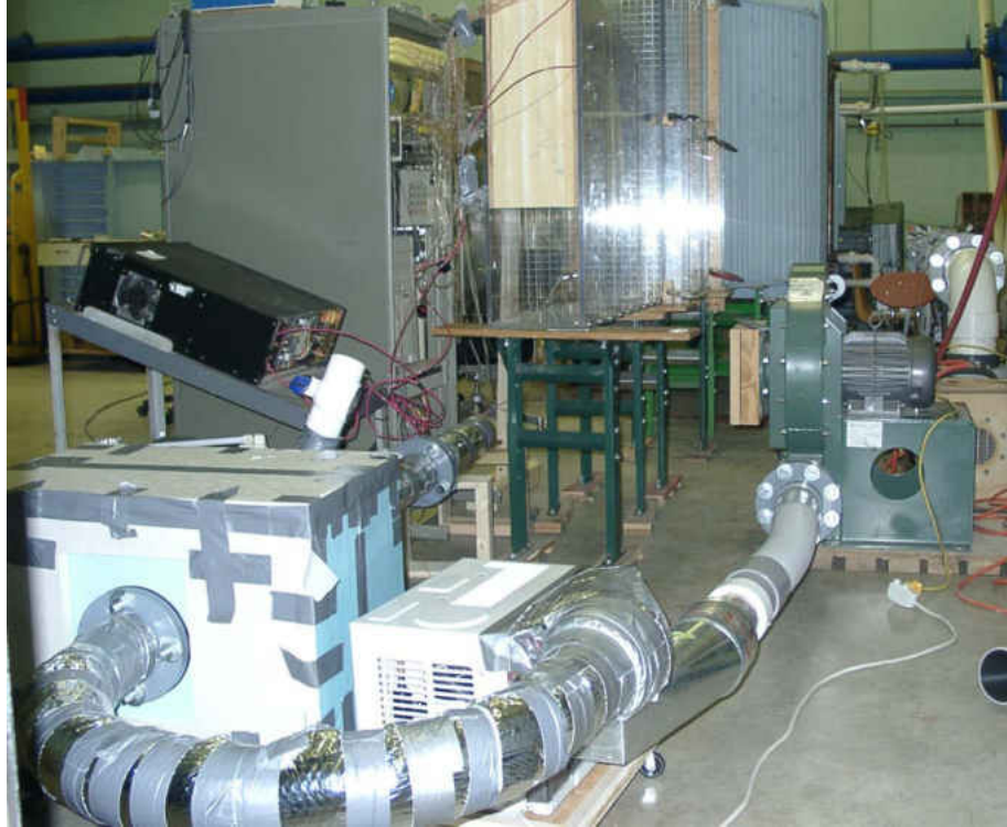
Figure 41. Blower, ac unit, thermal inertia box, orifice plate, and power supply.
