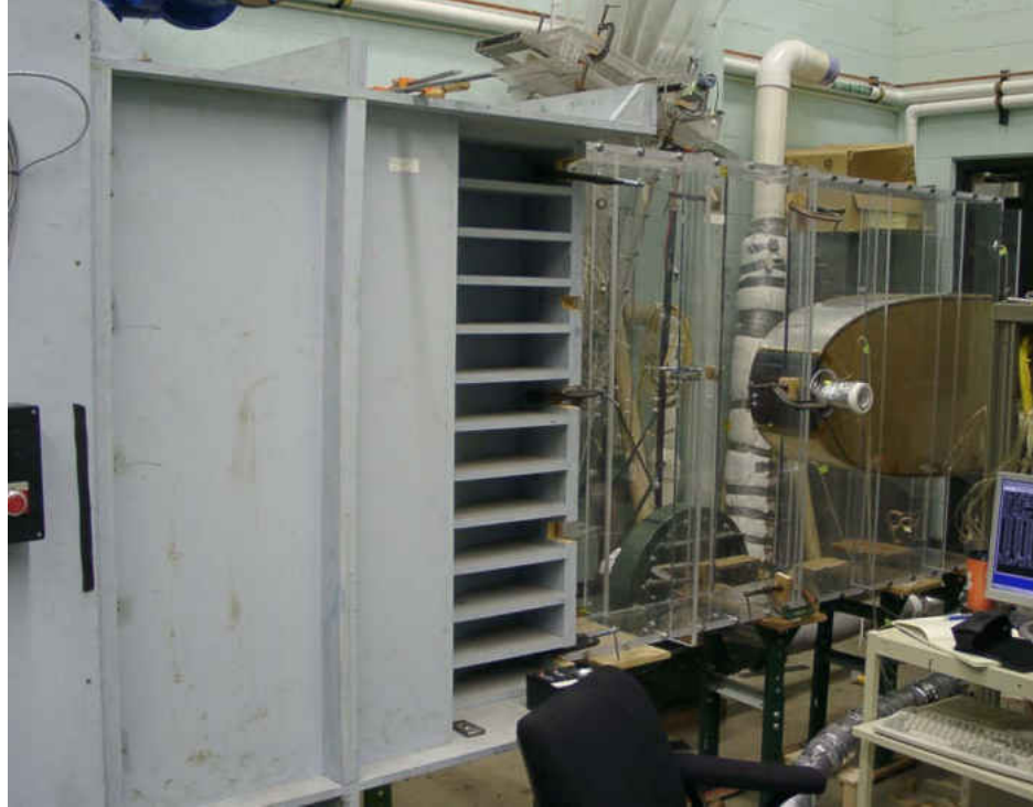
Figure 47. Large cylindrical test section, mock aero-combustor with spool.
