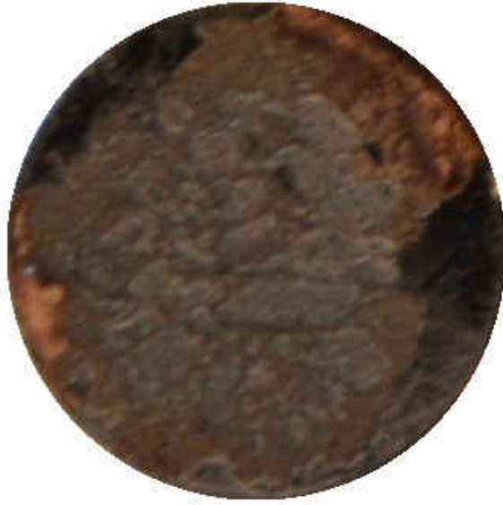
Figure D. 51: Experiment 26 run 14 fracture surface 1.
