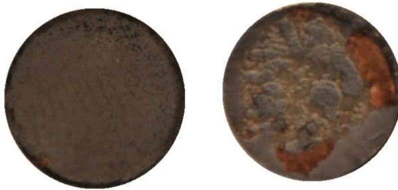
Figure 3. 5: left image is of a 25µm foil sample and the image on the right is of a 250µm sample. These images display the differences in fracture surface of the samples.
