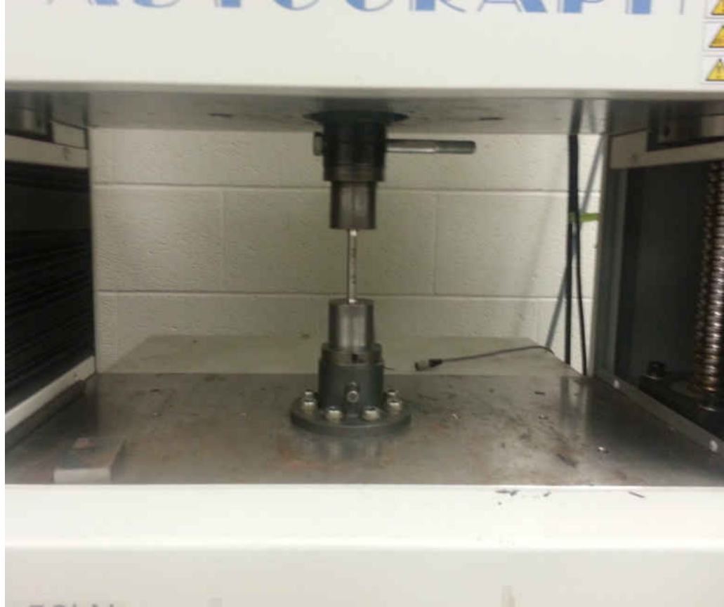
Figure 2.15: Shimadzu AG-IS Universal Testing Machine with round specimen tensile grips
