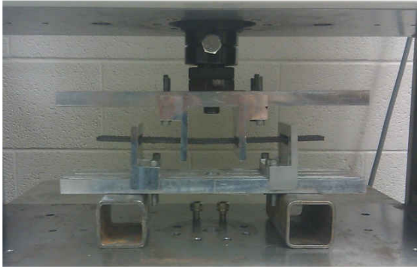
Figure 23. Static test setup with clamped four-point bending fixture.
