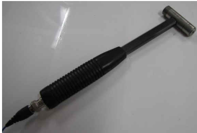
Figure 46. PCB Piezotronics 086C03 impact hammer used for excitation.
