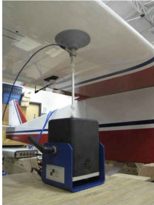
Figure 9. The shaker setup with stinger, load cell, and suction cup.
