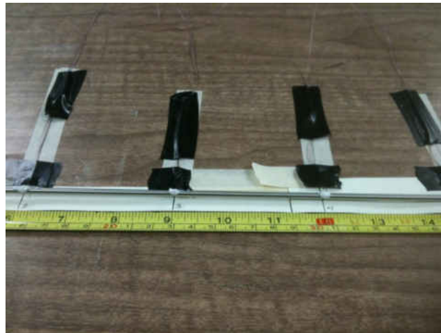
Figure 3.10. Thermocouple wire tip cemented to the test section outer wall with the help of Omega bond cement.
