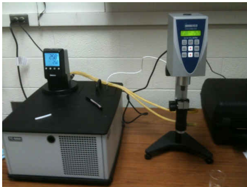
Figure 3.2. DV II+Pro Extra Brookfield viscometer connected to the TC-550MX temperature bath.
