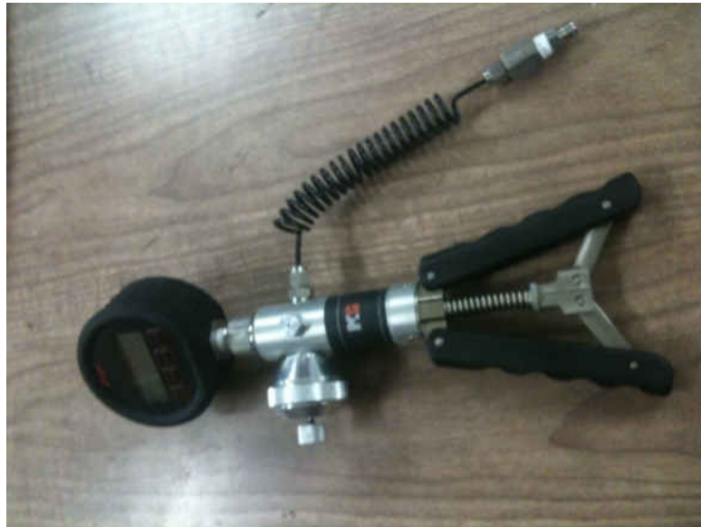
Figure 3.16 A meterk hand pump for calibration of the pressure transducers.
