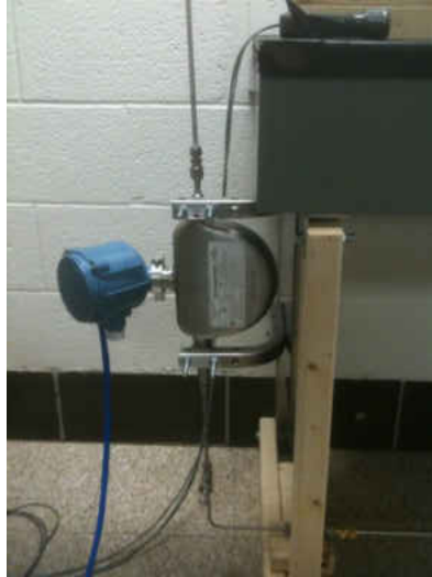
Figure 3. 7 Micro Motion mass flow sensor connected to a 1700R transmitter.
