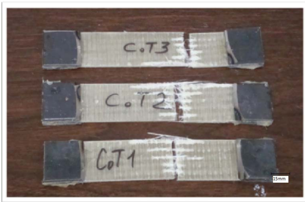
Fig.16 Characteristic failure pattern of E-glass/Polyester composite coupons after uniaxial tensile loading in transverse direction
