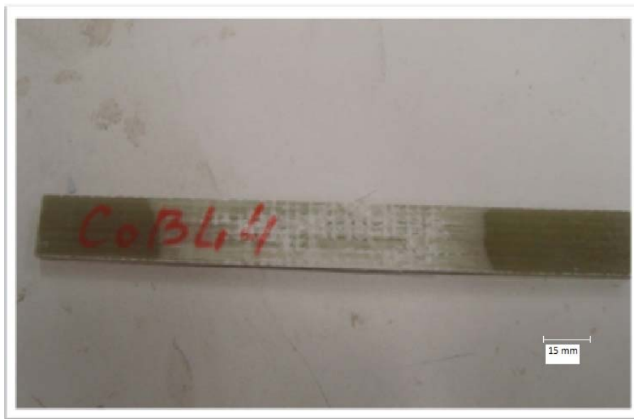
Fig.18 Typical failure of E-glass/Polyester composite beams in four-point bending in longitudinal direction
