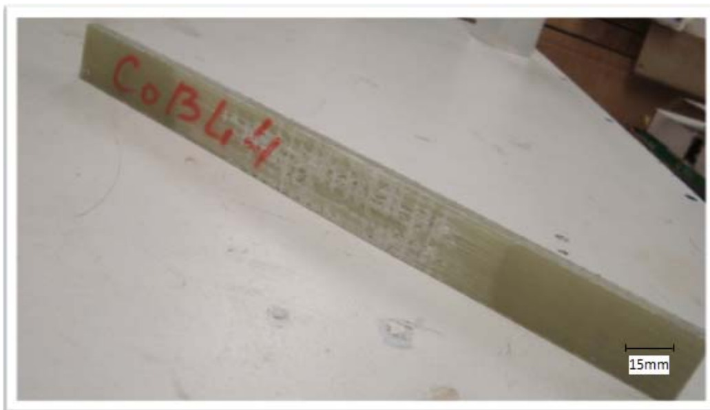
Fig.23 Failure of E-glass/Polyester composite beams in four-point bending in longitudinal direction
