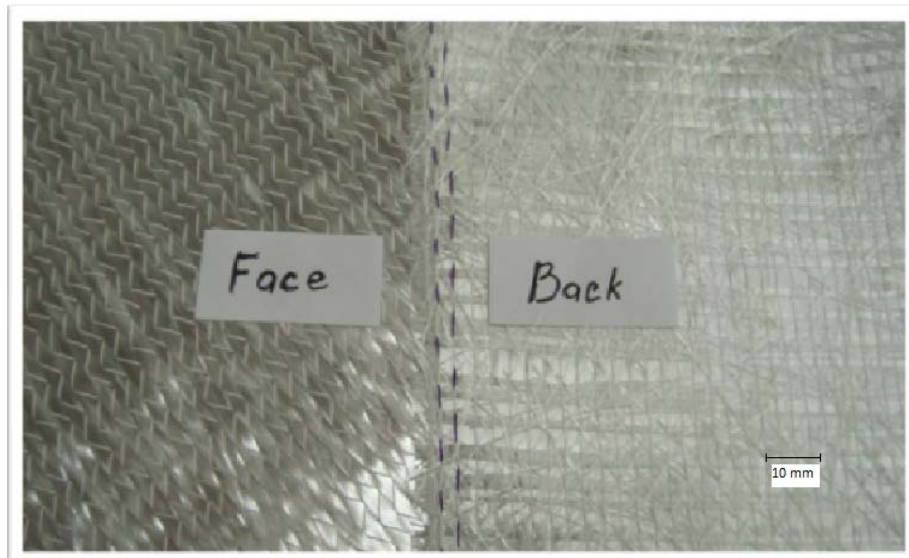
Fig.3 E-glass fiber chopped strand mat
