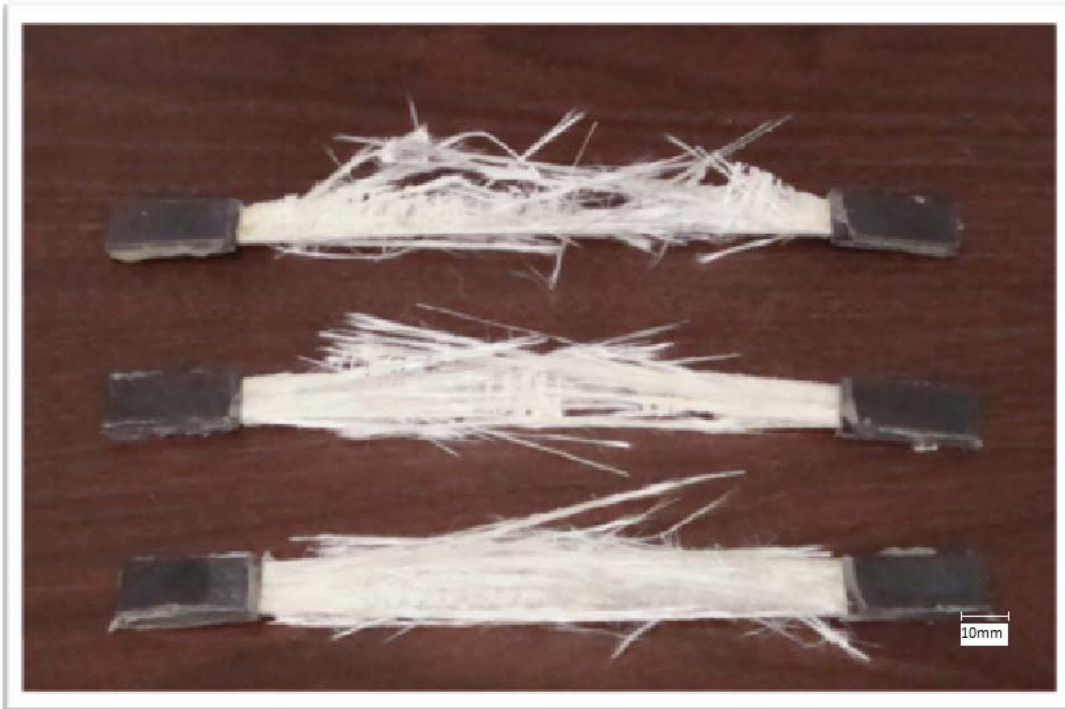
Fig.14 Characteristic failure pattern of E-glass/Polyester composite coupons after uniaxial tensile loading along the fiber direction
