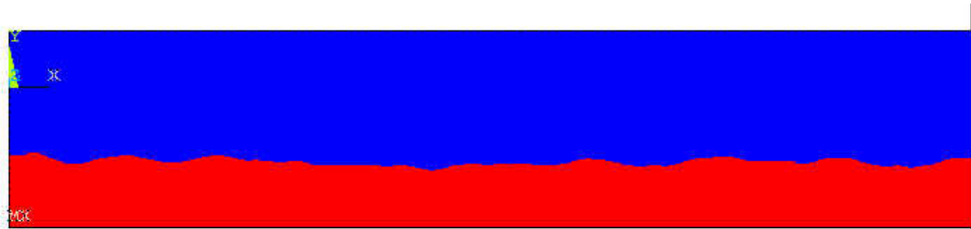
Figure 32: Time step 605, relative high displacement, Flotran volume fraction contour plot, 150 Hz case
