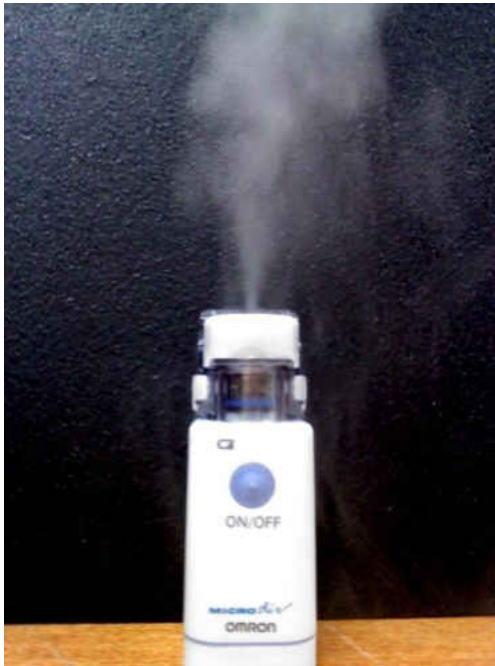
Figure 4: Omron Micro Air operating without inhalation assist tube Existing Theory of Operation
