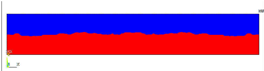
Figure 28: Full development of standing surface waves
