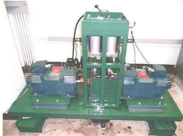
Figure 4 First generation sliding rolling contact fatigue tester [10]
