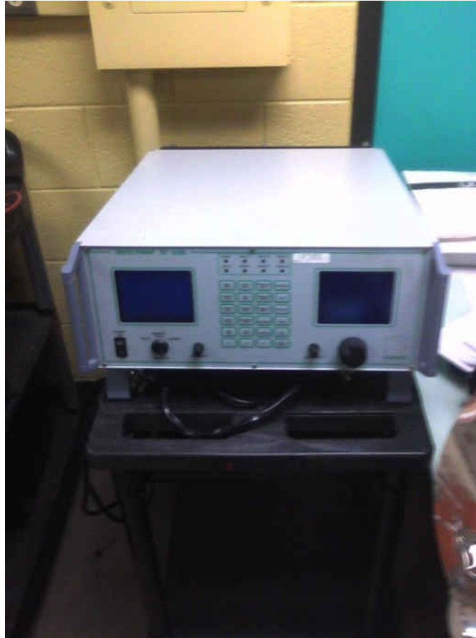
Figure 27 Foerster Defectomat EZ 2.828 Eddy Current Detection Device
