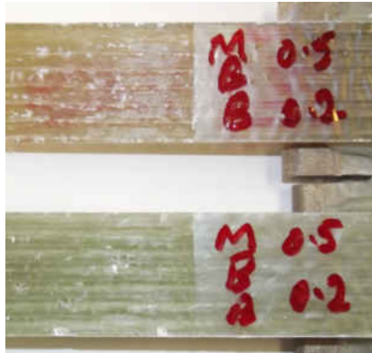
(e) Partial ply MB-B G_{II}/G=0.2
