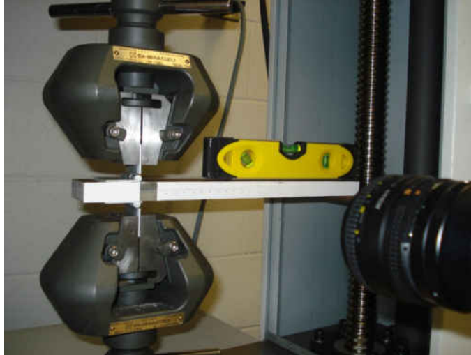
Figure 2.6. Experimental set-up for DCB testing
