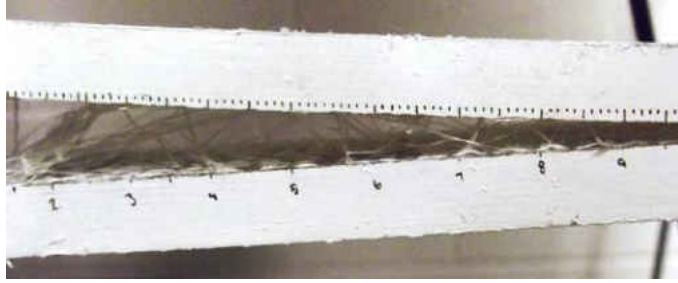
Figure 2.10. Fiber bridging in case of MB-A (main blade resin)
