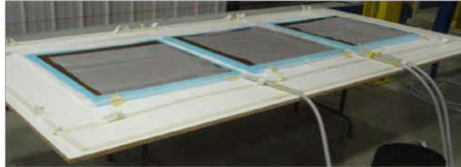
Figure 2.2. VARTM set-up before infusion
