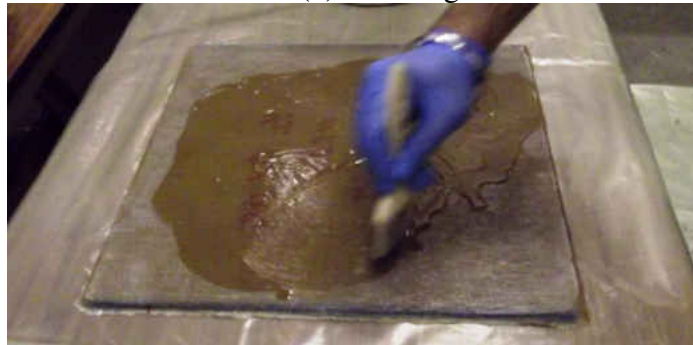
4.2 (c) Repair surface preparation
