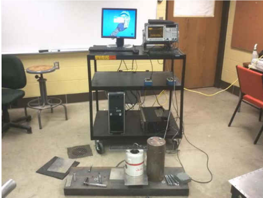
Figure 6.18: The Experimental Setup for the Beam with Sensor on Top
