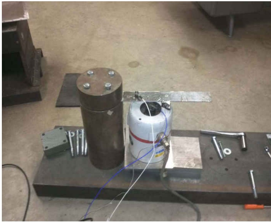
Figure 6.17: Side View of the Cantilevered Beam Setup
