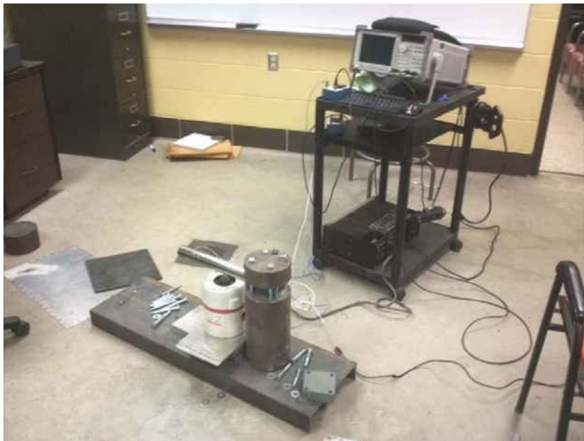
Figure 6.21: The Experimental Setup for the Pipe with Sensor on Top
