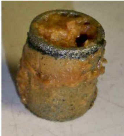
Figure 97. Fat-like residue on stainless steel filter during sub-cracking temperatures
