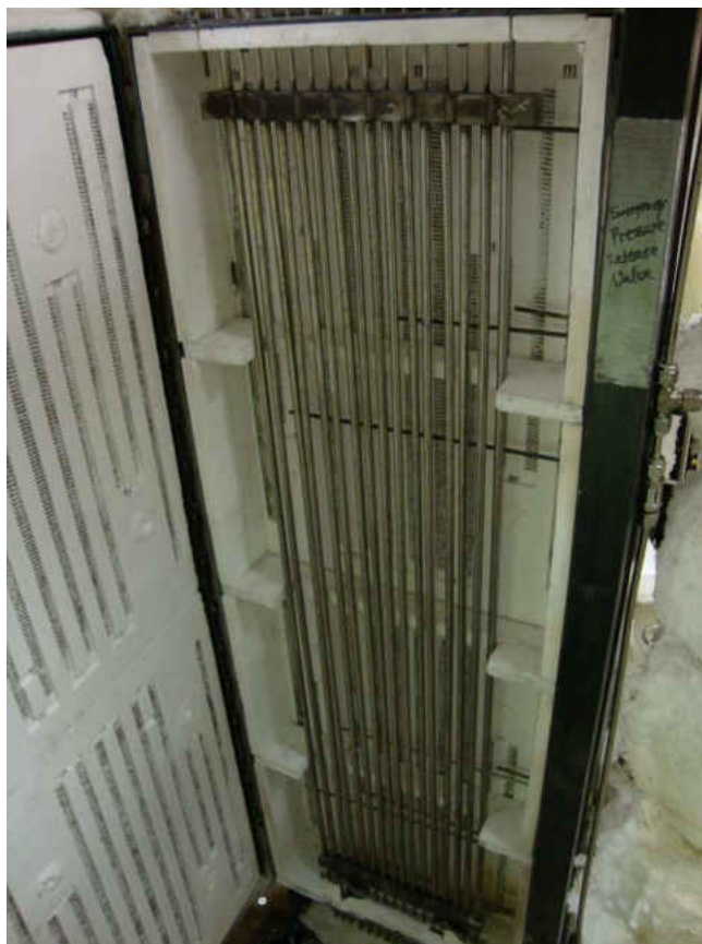
Figure 32. Bench-scale TCR photograph of cracking tubes
