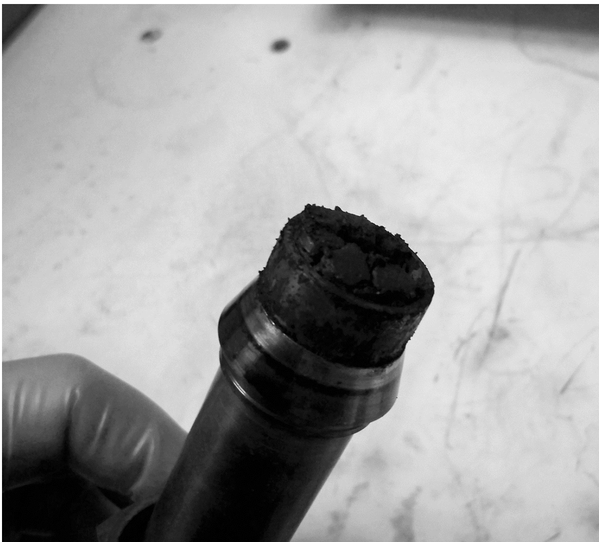
Figure 91. Coked bed of Ni/SiO 2 55 catalyst
